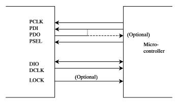
Figure 6. Microcontroller interface
