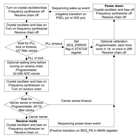
Figure 19. Automatic power-up sequencing flow chart
