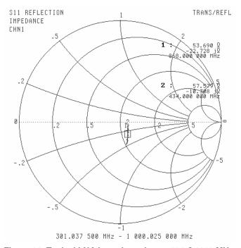
Figure 26. Typical LNA input impedance, 200 ñ 1000 MHz
