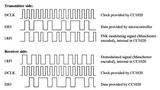
Figure 10. Synchronous Manchester encoded mode (SEP\_DI\_DO = 0)
