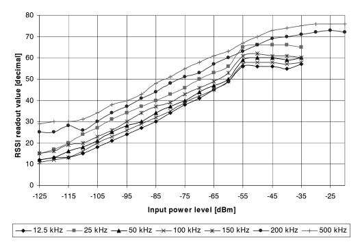
Figure 14. Typical RSSI value vs. input power for some typical channel spacings, 433 MHz
