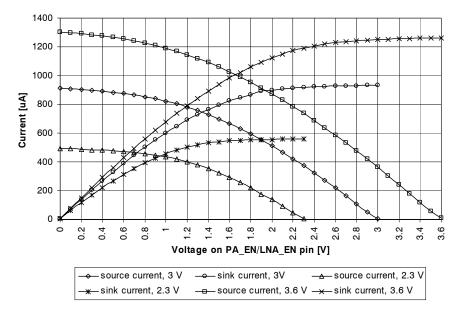
Figure 35. Typical PA\_EN and LNA\_EN pin drive
