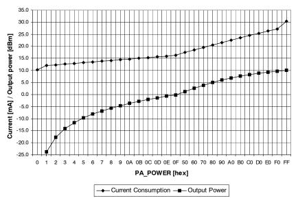
Figure 23. Typical output power and current consumption, 433 MHz
