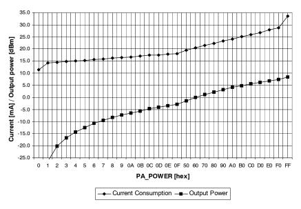
Figure 24. Typical output power and current consumption, 868 MHz
