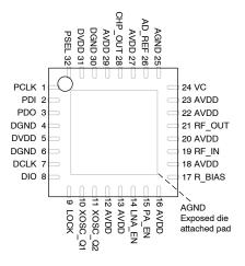
Figure 1. **CC1020** package (top view)
