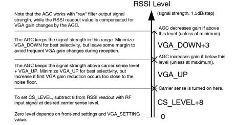
Figure 18. Relationship between RSSI, carrier sense level, and AGC settings CS\_LEVEL, VGA\_UP and VGA\_DOWN
