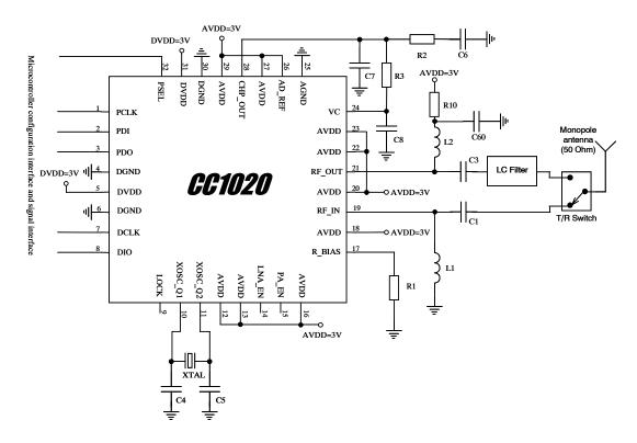
Figure 3. Typical application and test circuit (power supply decoupling not shown)
