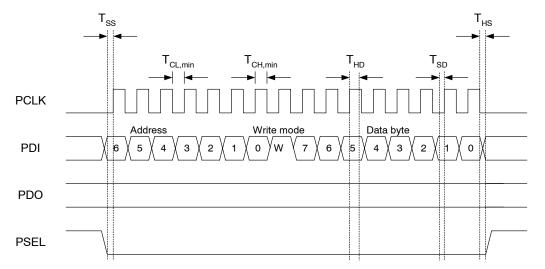
Figure 7. Configuration registers write operation
