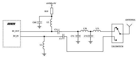
Figure 25. Input/output matching network
