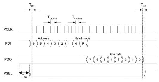
Figure 8. Configuration registers read operation
