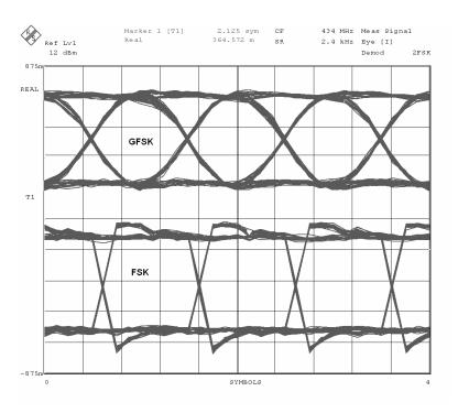
Figure 21. FSK vs. GFSK eye diagram. 2.4 kBaud, NRZ, ±2.025 kHz frequency deviation
