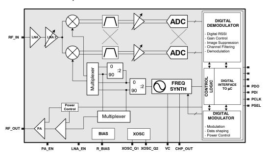
Figure 2. **CC1020** simplified block diagram
