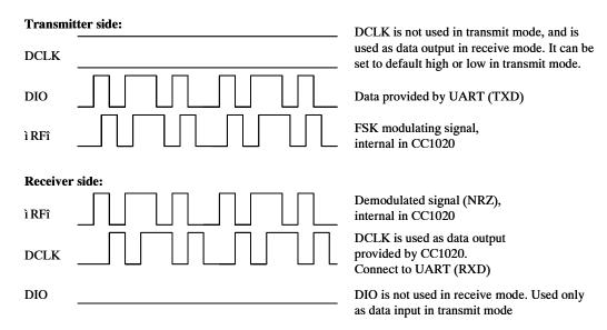
Figure 11. Transparent Asynchronous UART mode (SEP\_DI\_DO = 1)
