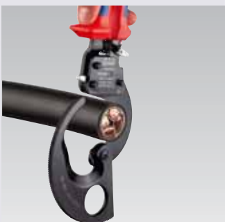
95 31 280: large cutting capacity: maximum 52 mm dia. / 380 mm 2
