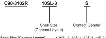
Shell Size (Contact Layout): 10SL-3, 10SL4, 12S-3, 14S-2 and 14S-6.Contact Gender: S = Female and P = Male.
