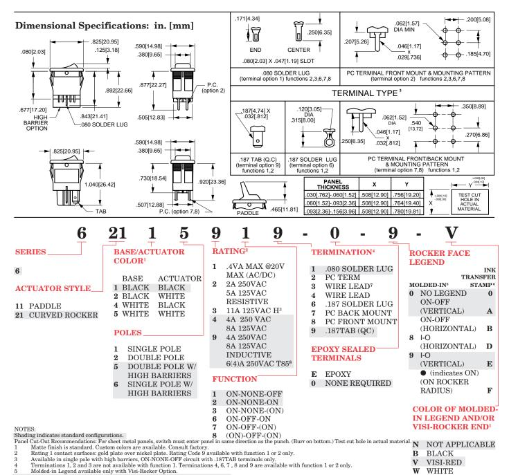
White is standard with dark actuators; black is standard with light actuators. Termination 3 available with rating 2 only - 18 gauge wire used. Rating 9 using Termination 1 or 2 is rated T55 only.
