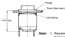
Note: 1. Recommended panel thickness: 1 to 1.6 mm
