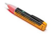
The next generation VoltAlert<sup>™</sup> ac voltage testers from Fluke are easy to use - just touch the tip to a terminal strip, outlet, or cord. When the tip glows red and the unit beeps, you know there's voltage present. Electricians, maintenance, service, safety personnel, and homeowners can quickly test for energized circuits at work or in the home.
