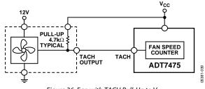
Figure 36. Fan with TACH Pull-Up to V.cc
