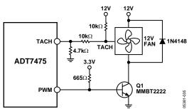
Figure 32. Driving a 3-Wire Fan Using an NPN Transistor
