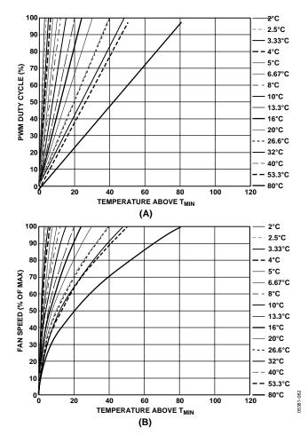
Figure 56. TRANGE vs. Actual Fan Speed (not PWM drive) Profile
