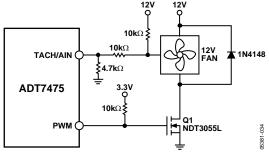
Figure 31. Driving a 3-Wire Fan Using an N-Channel MOSFET
