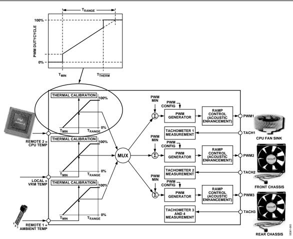
Figure 59. How T<sub>THERM</sub> Relates to Automatic Fan Control
