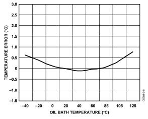
Figure 11. Internal Temperature Error vs. ADT7475 Temperature
