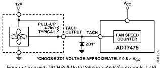
Figure 37. Fan with TACH Pull-Up to Voltage > 3.6 V (for example, 12 V) Clamped with Zener Diode
