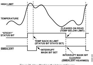
Figure 26. How Masking the Interrupt Source Affects SMBALERT Output
