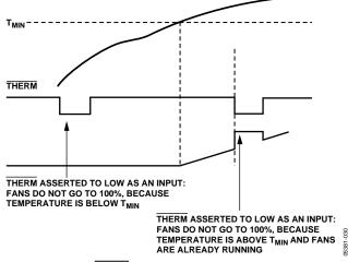
Figure 27. Asserting THERM Low as an Input in Automatic Fan Speed Control Mode
