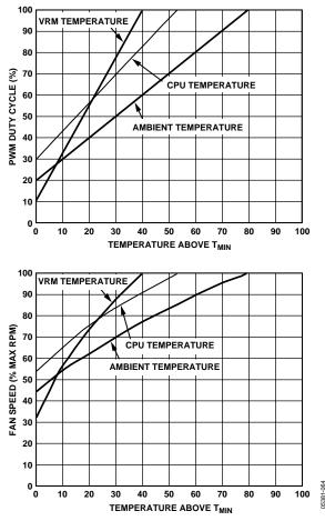
Figure 58. T<sub>RANGE</sub> and % Fan Speed Slopes for VRM, Ambient, and CPU Temperature Channels
