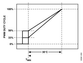
Figure 53. Adjusting PWM<sub>MIN</sub> Changes the Automatic Fan Control Slope
