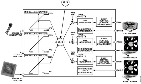
Figure 46. Assigning Temperature Channels to Fan Channels
