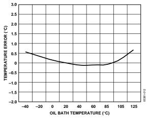
Figure 12. Remote Temperature Error vs. ADT7475 Temperature
