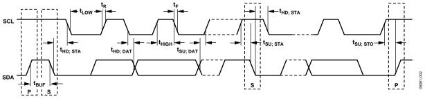
Figure 2. Serial Bus Timing Diagram
