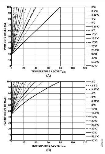
Figure 57. T<sub>RANGE</sub> and % Fan Speed Slopes with PWM<sub>MIN</sub> = 20%
