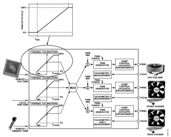
Figure 48. Understanding the T<sub>MIN</sub> Parameter
