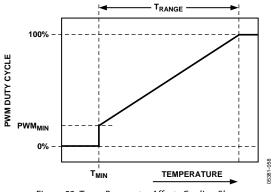
Figure 52. T<sub>RANGE</sub> Parameter Affects Cooling Slope
