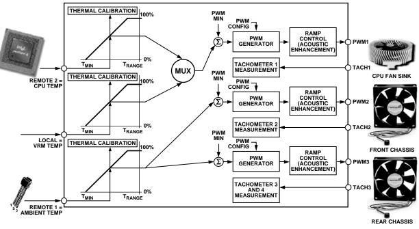
Figure 47. Mux Configuration Example
