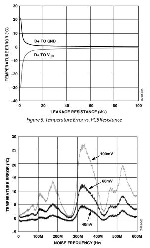
*Figure 6. Remote Temperature Error vs. Common-Mode Noise Frequency*
