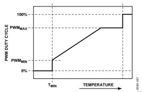
Figure 51. PWM<sub>MAX</sub> Determines Maximum PWM Duty Cycle below the THERM Temperature Limit
