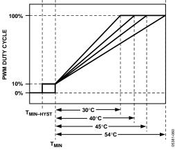
Figure 54. Increasing TRANGE Changes the AFC Slope
