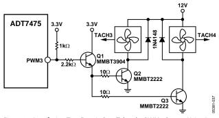
Figure 34. Interfacing Two Fans in Parallel to the PWM3 Output Using Low Cost NPN Transistors
