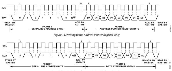
Figure 16. Reading Data from a Previously Selected Register
