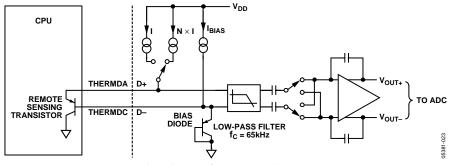
Figure 21. Signal Conditioning for Remote Diode Temperature Sensors
