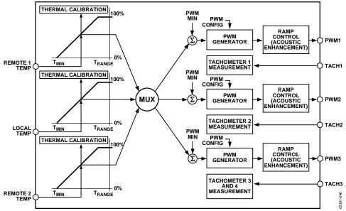
Figure 42. Automatic Fan Control Block Diagram
