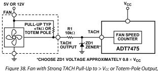
Figure 38. Fan with Strong TACH Pull-Up to  $> V_{CC}$  or Totem-Pole Outpulling Clamped with Zener and Resistor
