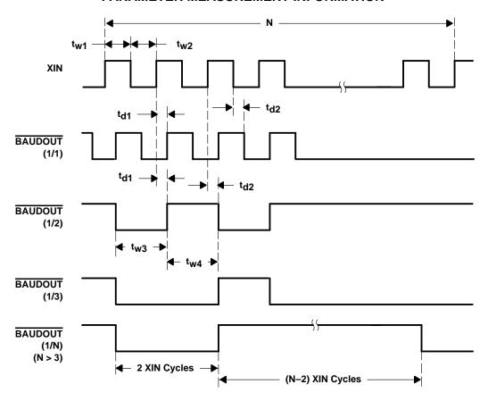
Figure 5. Baud Generator Timing Waveforms
