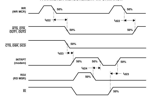
**Figure 16. Modem Control Timing Waveforms**
