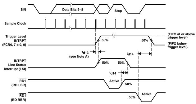
NOTE A: For a time-out interrupt,  $t_{d13} = 9$  RCLKs.
