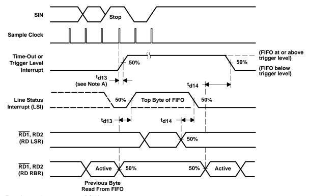
NOTE A: For a time-out interrupt,  $t_{d13} = 9$  RCLKs.
