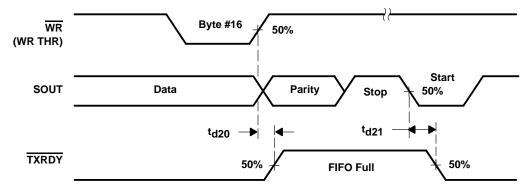
Figure 15. Transmitter Ready (TXRDY) Waveforms, FCR0 = 1 and FCR3 = 1 (Mode 1)
