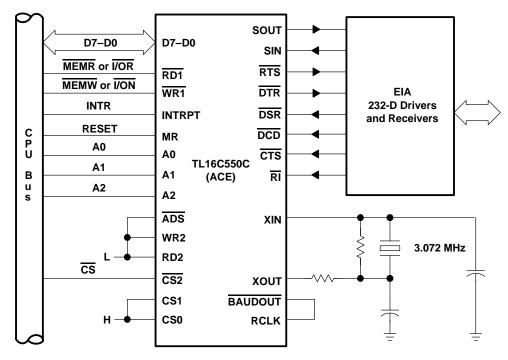
Figure 20. Basic TL16C550C Configuration
