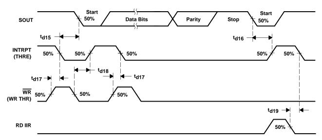
**Figure 13. Transmitter Timing Waveforms**
