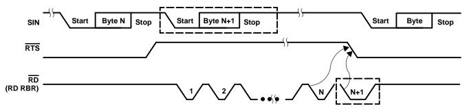
NOTES: A. N = RCV FIFO trigger level (1, 4, or 8 bytes)
