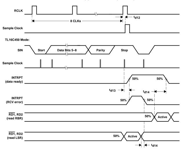
Figure 8. Receiver Timing Waveforms
