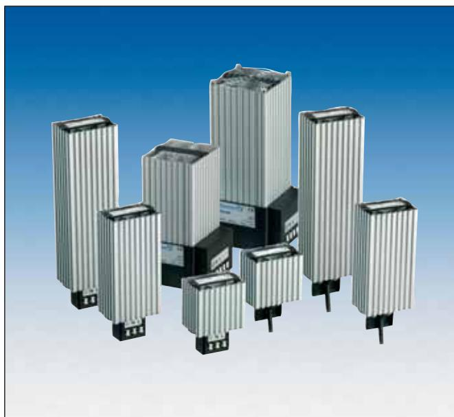
Heat generated by electrical equipment operating under load will prevent the accumulation of condensation. After the equipment has been switched off however it cools down and gradually adapts to the ambient temperature, thus dropping below the dew point. This is the signal that triggers the radiant heater! These sources of heat prevent the formation of condensation by raising the internal temperature a few degrees above the ambient temperature.
