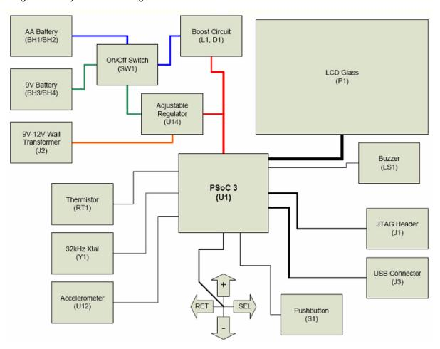
PSoC 3 LCD Segment Drive EVK showcases PSoC's LCD segment drive capability by driving a custom glass with 448 segments (16 common lines by 28 segments lines). This kit also highlights the PSoC's superior ability to integrate high performance digital and analog peripherals by integrating the accelerometer, thermistor, Real Time Clock, CapSense, and buzzer.
