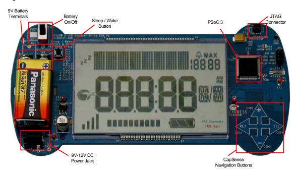
Operator entries are made using the four CapSense buttons that are labeled: SEL, "+", "-", and RET.
