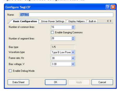
Figure 5-25. Segment LCD Configuration: Basic Tab
