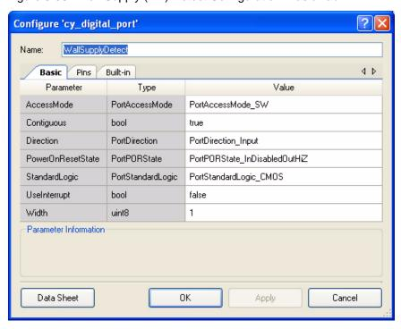
Figure 5-39. Wall Supply (Vin) Detect Configuration: Pins Tab
