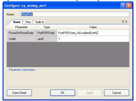
Figure 5-4. Thermistor Reference Analog Port Configuration: Basic Tab
