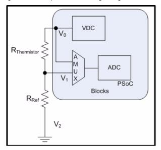
This setup significantly removes gain and offset errors from the resistance calculation.
