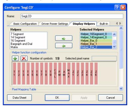
It includes remaining icon pixels: four large decimal points, large colon, slash, bell, MAX, AM, PM, small decimal points, and small colon).
