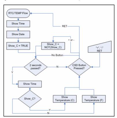
Figure 5-58. Clock Show Time and Date/Temperature Flow
