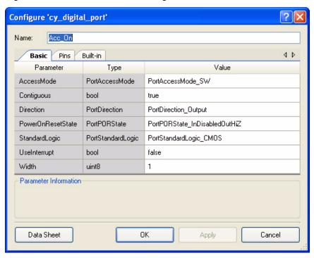
Figure 5-43. Accelerometer On Configuration: Pin Tab
