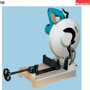
1650W TCT circular saw. Spark free, cold clean cut five times faster than abrasive cut-off machines. Maximum cut at  $90^\circ$  115mm diameter, at  $45^\circ$  90mm diameter. Fitted with electric brake and quick release vice.
