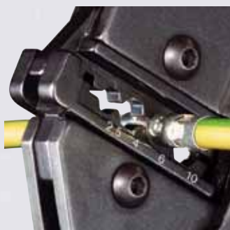
Crimp System Plier 97 43 200 with crimp profile 97 49 30 for non-insulated butt connectors
