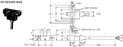
\* Three-conductor, thirteen, 0.12-wire cable (2-m long, 3.5 dia.)
