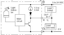
Note: Voltage output (when the sensor is connected to a transistor circuit).
