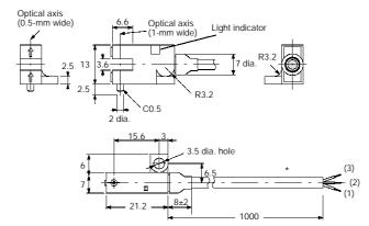
\* Three-conductor, thirteen, 0.12-wire cable (1-m long, 3.5 dia.)
