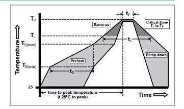
Wave Soldering Parameters
