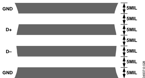
Figure 29. Arrangement of Signal Tracks
