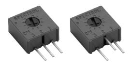
The Model 63 cermet trimmer is available in several pin configurations for top or side adjustment and with a choice of Knob styles for finger setting. Quick adjustment is achieved with multi-finger wiper and the standard resistance range is between 100  $\Omega$  and 2 M $\Omega$  with a tolerance of  $\pm$  10 %.
