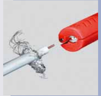
Stripping the conductor of a Coax-cable
