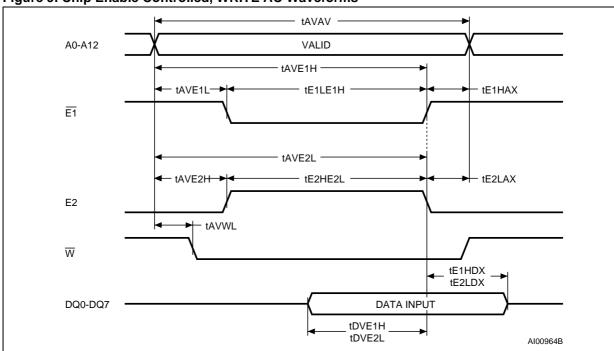
Figure 9. Chip Enable Controlled, WRITE AC Waveforms
