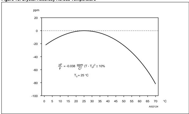
Figure 11. Clock Calibration
