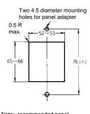
Note: recommended panel thickness is 1 to 3.2 mm..
