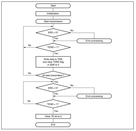
Figure 15.28 Example of Transmission Processing Flow
