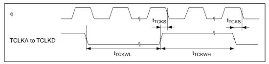
Figure 24.37 TPU Clock Input Timing
