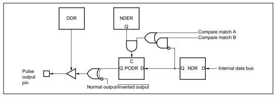
Figure 12.6 Non-Overlapping Pulse Output
