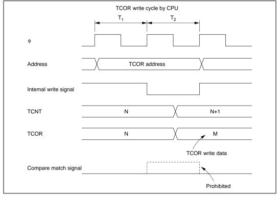
Figure 13.12 Contention between TCOR Write and Compare Match
