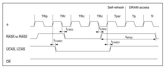
Figure 24.22 Self-Refresh Timing (Return from Software Standby Mode: RAST = 0)
