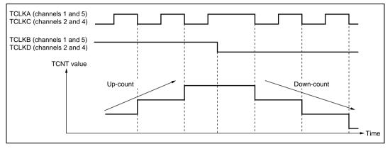
Figure 11.26 Example of Phase Counting Mode 2 Operation
