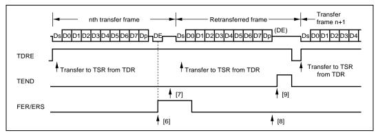
Figure 15.26 Retransfer Operation in SCI Transmit Mode
