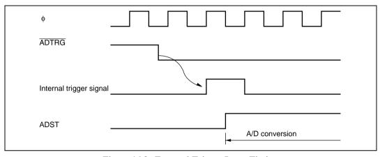
Figure 16.3 External Trigger Input Timing
