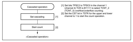
Figure 11.17 Cascaded Operation Setting Procedure
