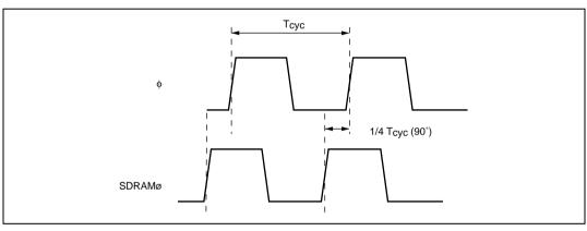
Figure 6.43 Relationship between  $\phi$  and SDRAM $\phi$  (when PLL frequency multiplication factor is  $\times 1$  or  $\times 2$ )
