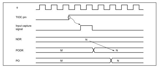
Figure 12.11 Pulse Output Triggered by Input Capture (Example)
