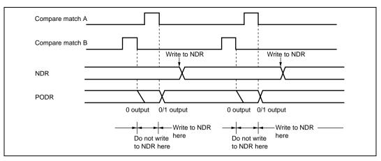
Figure 12.7 Non-Overlapping Operation and NDR Write Timing
