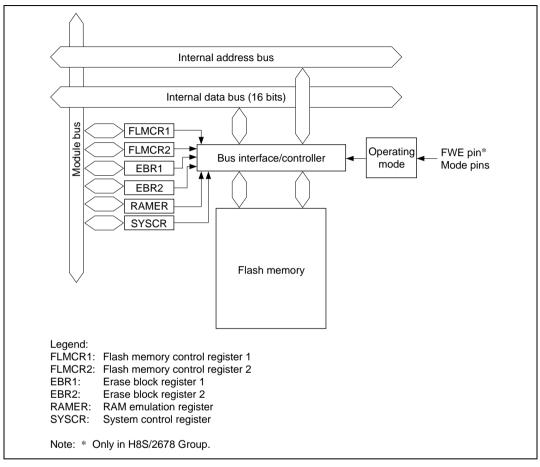
Figure 19.1 Block Diagram of Flash Memory
