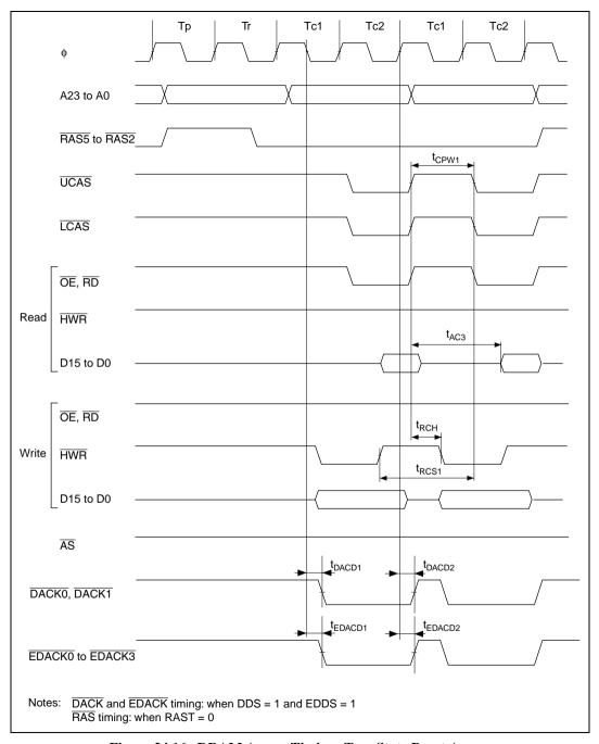
Figure 24.16 DRAM Access Timing: Two-State Burst Access
