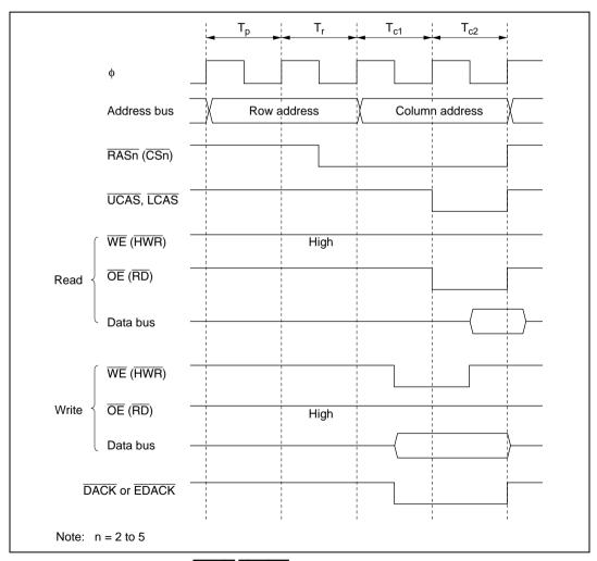
Figure 6.41 Example of  $\overline{DACK}/\overline{EDACK}$  Output Timing when DDS = 1 or EDDS = 1 (RAST = 0, CAST = 0)
