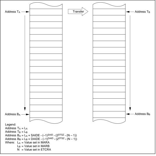
Figure 7.11 Operation in Normal Mode
