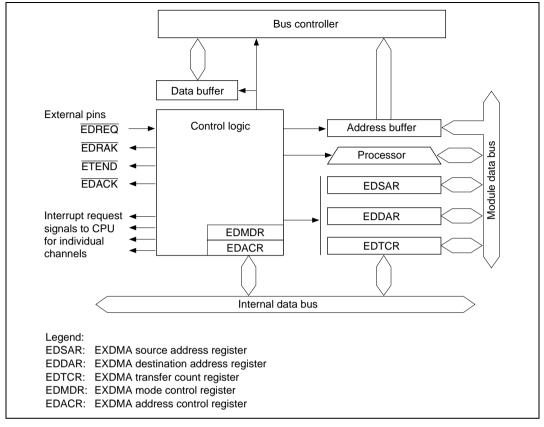
Figure 8.1 Block Diagram of EXDMAC
