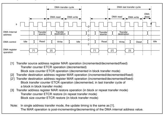
Figure 7.39 DMAC Register Update Timing
