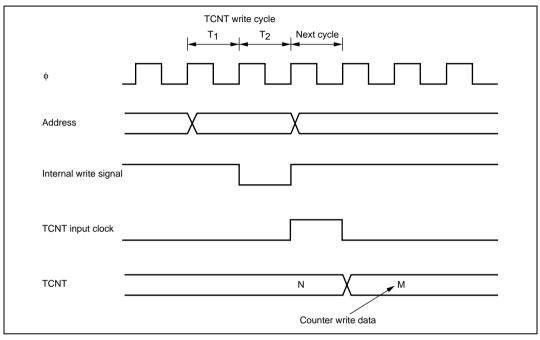
Figure 14.5 Contention between TCNT Write and Increment
