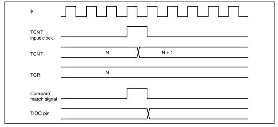
Figure 11.32 Output Compare Output Timing
