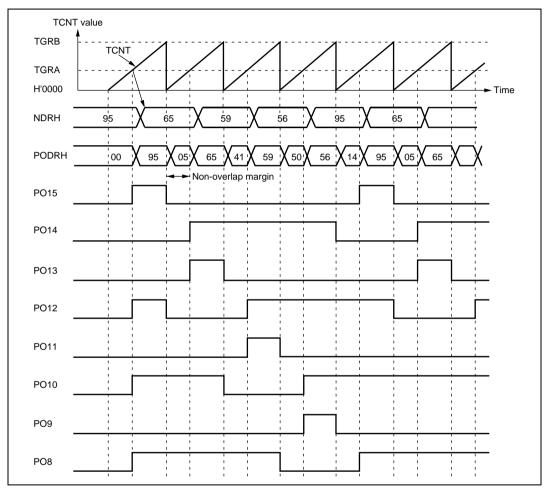
Figure 12.9 Non-Overlapping Pulse Output Example (Four-Phase Complementary)
