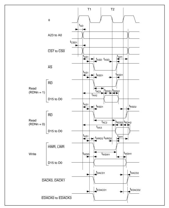
Figure 24.7 Basic Bus Timing: Two-State Access
