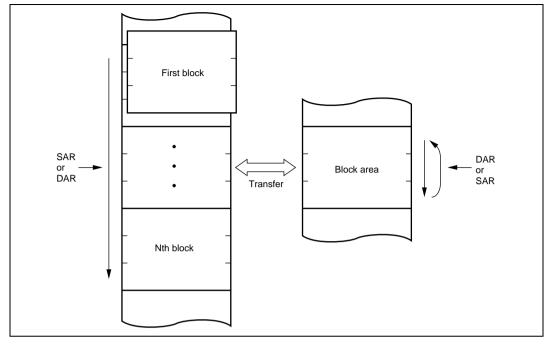
Figure 9.7 Memory Mapping in Block Transfer Mode
