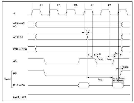
Figure 24.13 Burst ROM Access Timing: Two-State Burst Access
