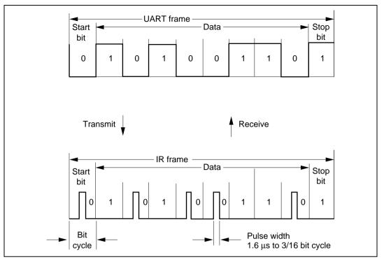
Figure 15.34 IrDA Transmit/Receive Operations
