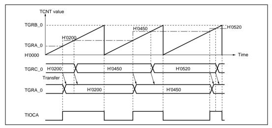
Figure 11.15 Example of Buffer Operation (1)
