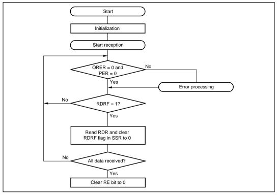
Figure 15.30 Example of Reception Processing Flow
