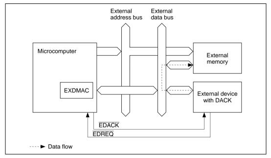
Figure 8.3 Data Flow in Single Address Mode
