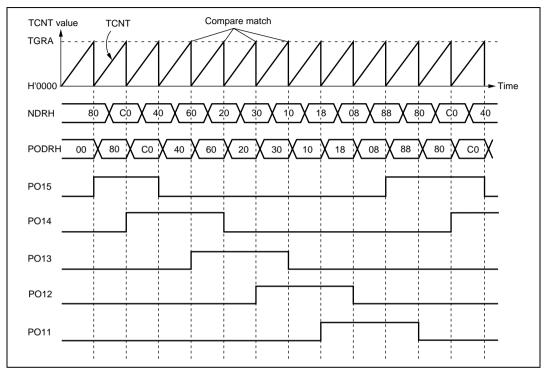
Figure 12.5 Normal Pulse Output Example (Five-Phase Pulse Output)
