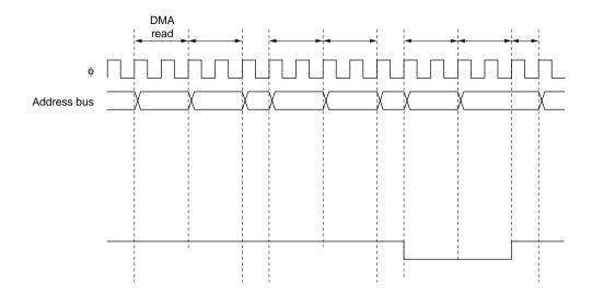
**Full Address Mode (Burst Mode):** Figure 7.20 shows a transfer example in which TEND output is enabled and word-size full address mode transfer (burst mode) is performed from external 16-bit, 2-state access space to external 16-bit, 2-state access space.
