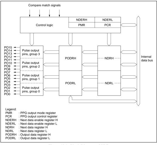
Figure 12.1 Block Diagram of PPG
