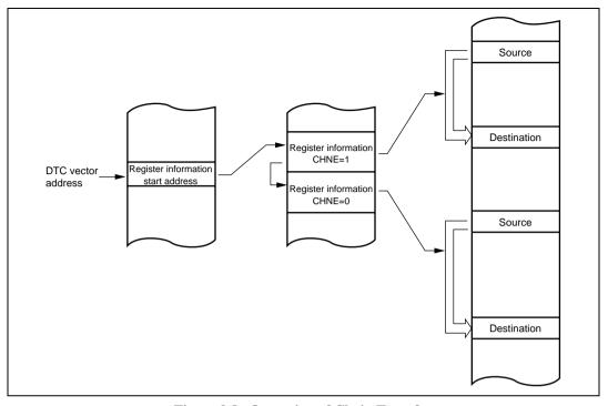
Figure 9.8 Operation of Chain Transfer
