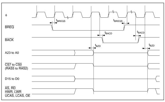
Figure 24.24 External Bus Release Timing
