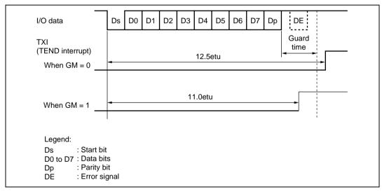
Figure 15.27 TEND Flag Generation Timing in Transmission Operation
