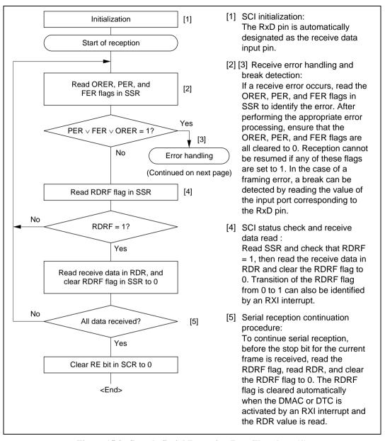
Figure 15.9 Sample Serial Reception Data Flowchart (1)
