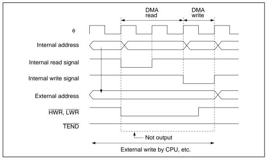
Figure 7.41 Example in Which Low Level Is Not Output at TEND Pin
