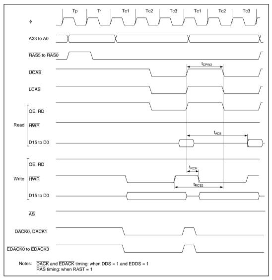
Figure 24.19 DRAM Access Timing: Three-State Burst Access
