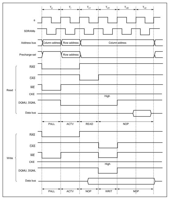
Figure 6.45 CAS Latency Control Timing (SDWCD = 0, CAS Latency 3)
