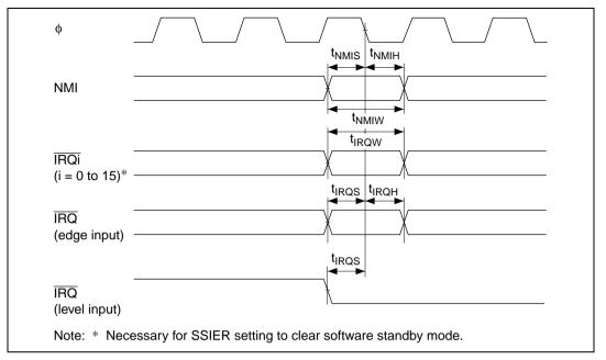
Figure 24.6 Interrupt Input Timing
