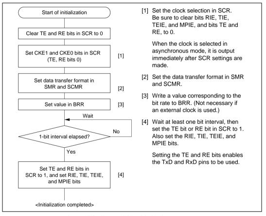
Figure 15.5 Sample SCI Initialization Flowchart
