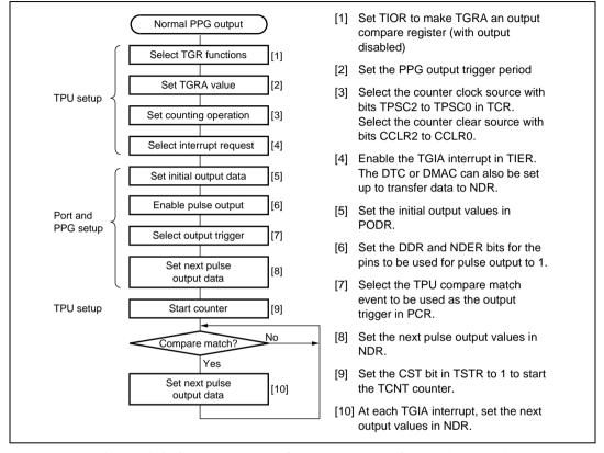
Figure 12.4 Setup Procedure for Normal Pulse Output (Example)
