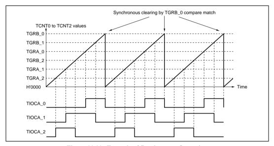
Figure 11.11 Example of Synchronous Operation
