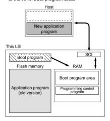
4. Writing new application program The programming control program transferred from the host to RAM is executed, and the new application program in the host is written into the
