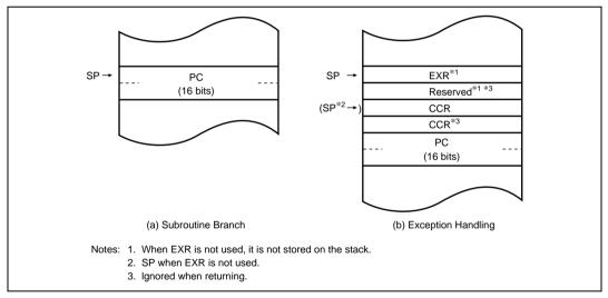
Figure 2.2 Stack Structure in Normal Mode
