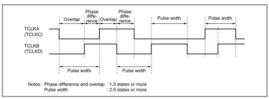
Figure 11.44 Phase Difference, Overlap, and Pulse Width in Phase Counting Mode
