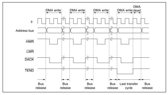
Figure 7.28 Example of Single Address Mode Transfer (Byte Write)
