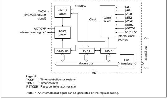
Figure 14.1 Block Diagram of WDT
