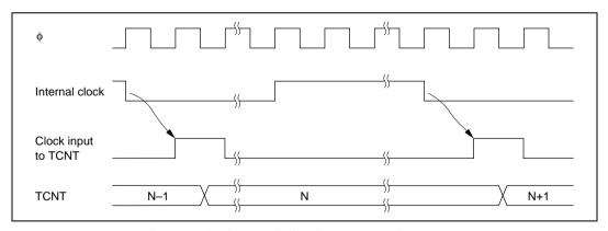
Figure 13.3 Count Timing for Internal Clock Input
