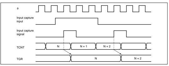
Figure 11.33 Input Capture Input Signal Timing
