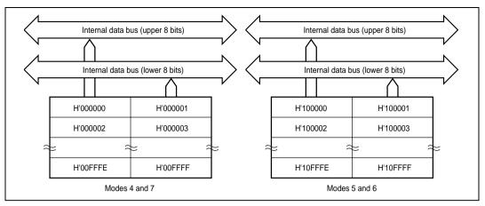
Figure 20.3 Block Diagram of 64-kbyte Masked ROM (HD6432673)
