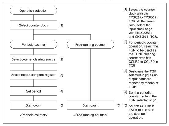
Figure 11.2 Example of Counter Operation Setting Procedure
