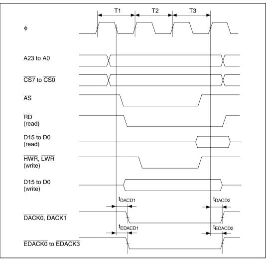
Figure 24.30 DMAC and EXDMAC Single Address Transfer Timing: Three-State Access
