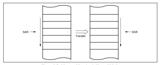
Figure 9.5 Memory Mapping in Normal Mode
