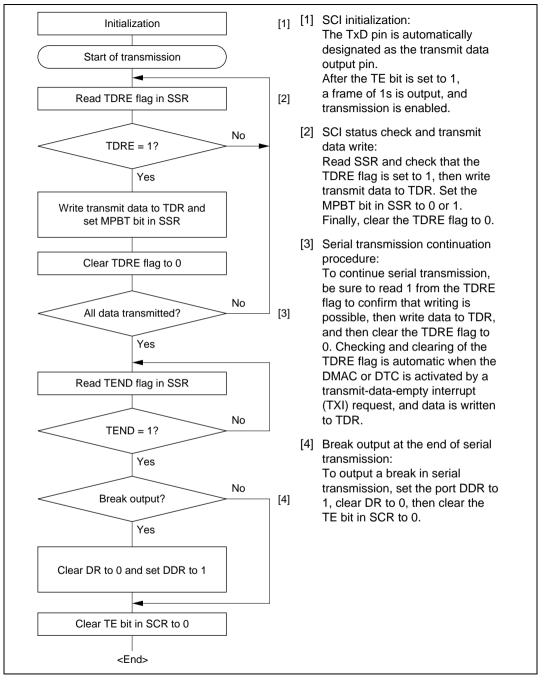
Figure 15.11 Sample Multiprocessor Serial Transmission Flowchart
