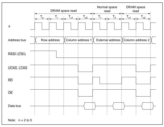
Figure 6.32 Example of Operation Timing in RAS Down Mode (RAST = 0, CAST = 0)
