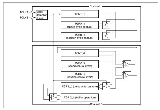
Figure 11.29 Phase Counting Mode Application Example
