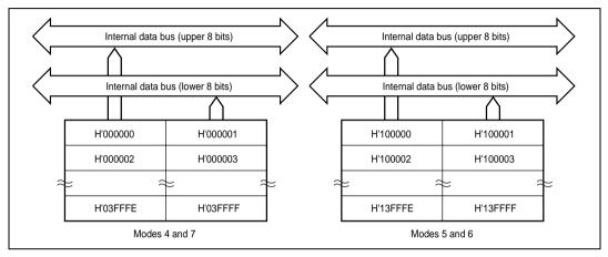
Figure 20.1 Block Diagram of 256-kbyte Masked ROM (HD6432676)
