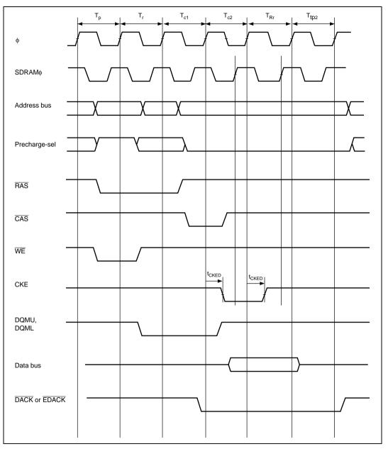
Figure 24.28 Read Data: Two-State Expansion (CAS Latency 2)
