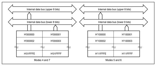
Figure 20.2 Block Diagram of 128-kbyte Masked ROM (HD6432675)
