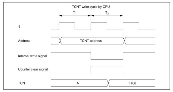
Figure 13.10 Contention between TCNT Write and Clear
