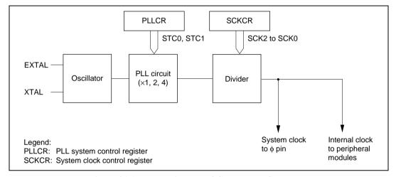
Figure 21.1 Block Diagram of Clock Pulse Generator
