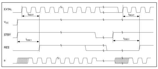
Figure 24.4 (1) Oscillation Stabilization Timing
