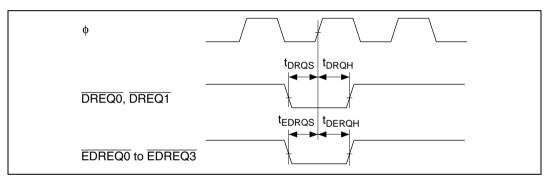
Figure 24.32 DMAC and EXDMAC DREQ/EDREQ Input Timing
