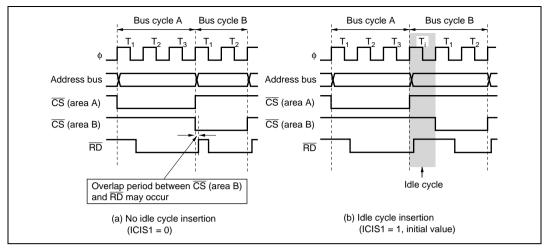
Figure 6.68 Relationship between Chip Select (CS) and Read (RD)
