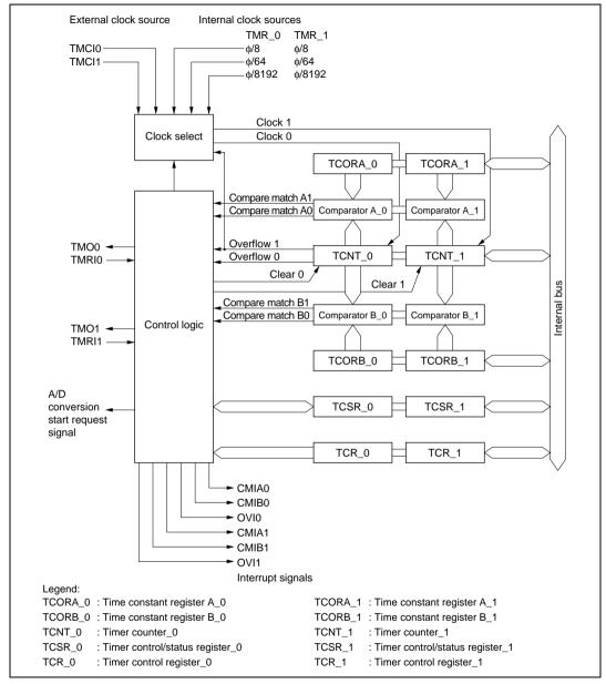
Figure 13.1 Block Diagram of 8-Bit Timer Module
