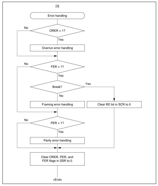
Figure 15.9 Sample Serial Reception Data Flowchart (2)
