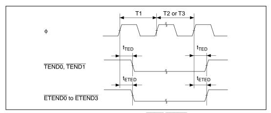
Figure 24.31 DMAC and EXDMAC TEND/ETEND Output Timing
