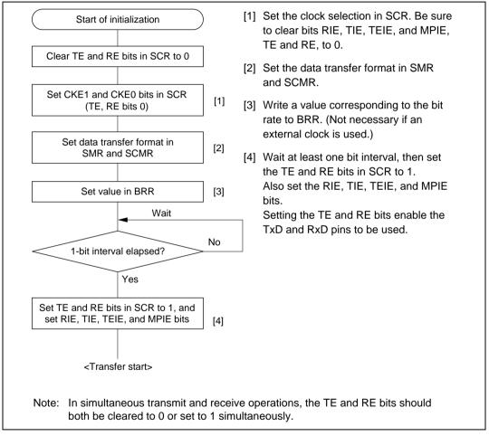
Figure 15.15 Sample SCI Initialization Flowchart
