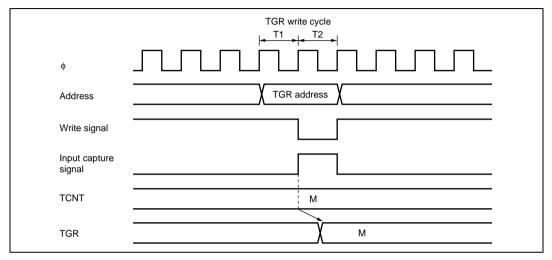
Figure 11.50 Contention between TGR Write and Input Capture
