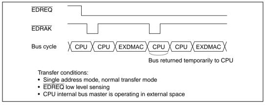
Figure 8.5 Example of Timing in Cycle Steal Mode
