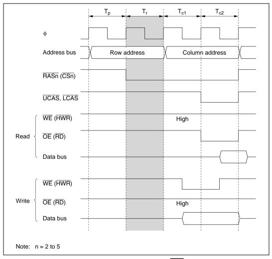
Figure 6.23 Example of Access Timing when  $\overline{RAS}$  Signal Goes Low from Beginning of  $T_r$  State (CAST = 0)
