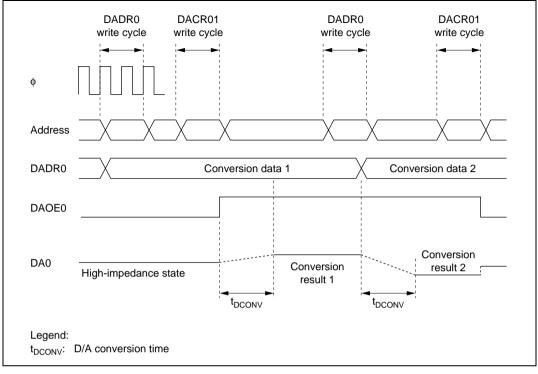
Figure 17.2 Example of D/A Converter Operation
