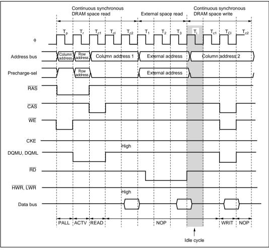
Figure 6.75 Example of Idle Cycle Operation in RAS Down Mode (Write after Read) (IDLC = 0, CAS Latency 2)
