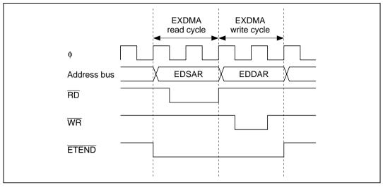
Figure 8.2 Example of Timing in Dual Address Mode
