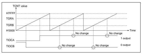
Figure 11.6 Example of 0 Output/1 Output Operation
