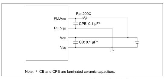
Figure 21.7 Recommended External Circuitry for PLL Circuit
