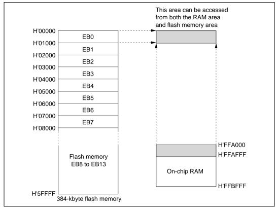
Figure 19.9 Example of RAM Overlap Operation
