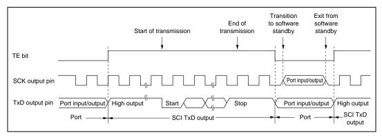
Figure 15.37 Port Pin States during Mode Transition (Internal Clock, Asynchronous Transmission)
