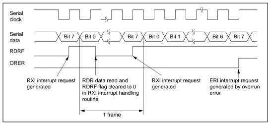
Figure 15.18 Example of SCI Operation in Reception
