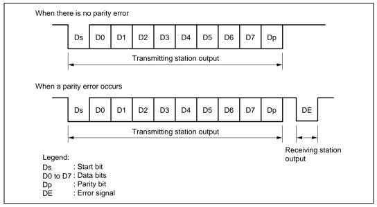
Figure 15.22 Normal Smart Card Interface Data Format
