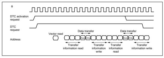
Figure 9.11 DTC Operation Timing (Example of Chain Transfer)
