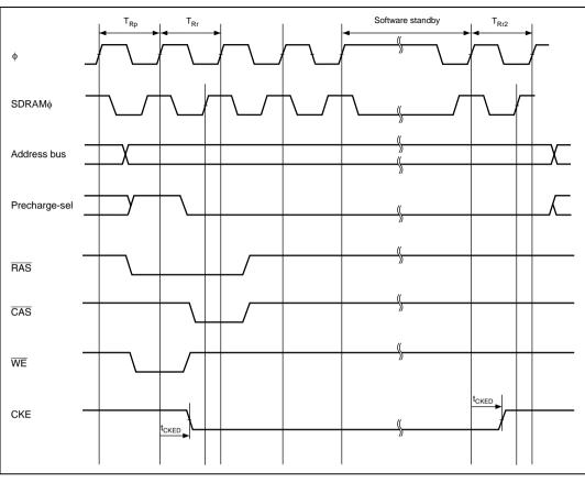
Figure 24.27 Synchronous DRAM Self-Refresh Timing
