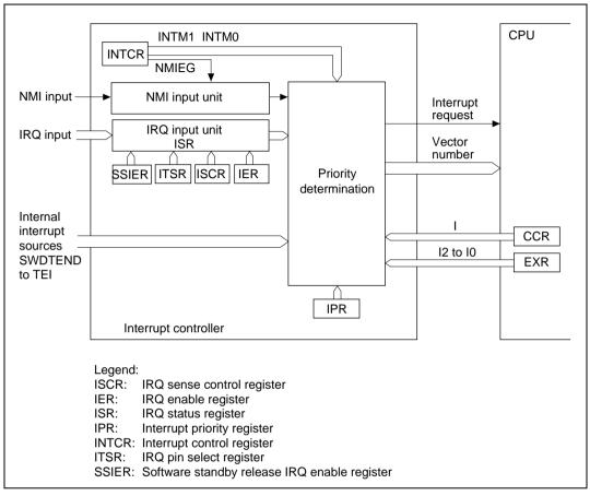
Figure 5.1 Block Diagram of Interrupt Controller
