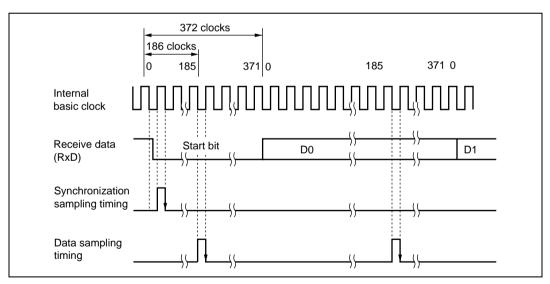
Figure 15.25 Receive Data Sampling Timing in Smart Card Mode (Using Clock of 372 Times the Bit Rate)
