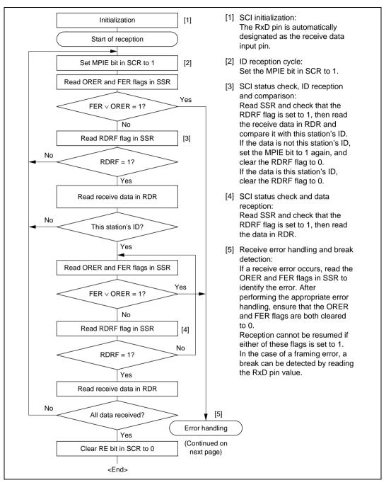
Figure 15.13 Sample Multiprocessor Serial Reception Flowchart (1)
