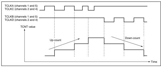
Figure 11.27 Example of Phase Counting Mode 3 Operation
