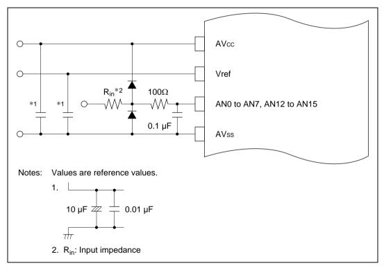
Figure 16.7 Example of Analog Input Protection Circuit
