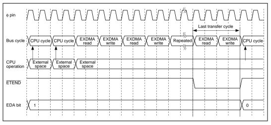
Figure 8.31 Auto Request/Burst Mode/Normal Transfer Mode (CPU Cycles/Dual Address Mode/BGUP = 0)
