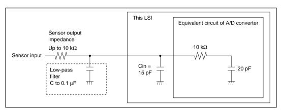
Figure 16.6 Example of Analog Input Circuit
