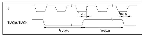
Figure 24.39 8-Bit Timer Clock Input Timing
