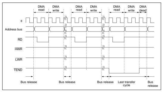
Figure 7.18 Example of Short Address Mode Transfer
