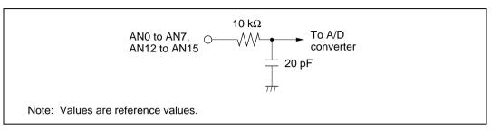
Figure 16.8 Analog Input Pin Equivalent Circuit
