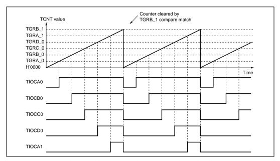
Figure 11.22 Example of PWM Mode Operation (2)
