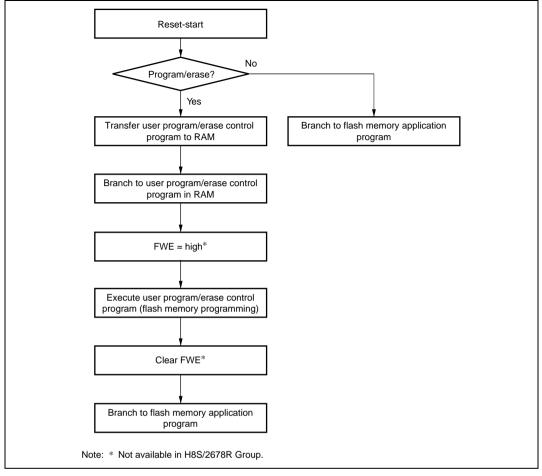
Figure 19.7 Programming/Erasing Flowchart Example in User Program Mode
