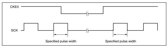
Figure 15.31 Timing for Fixing Clock Output Level
