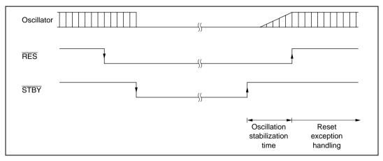
Figure 22.3 Hardware Standby Mode Timing
