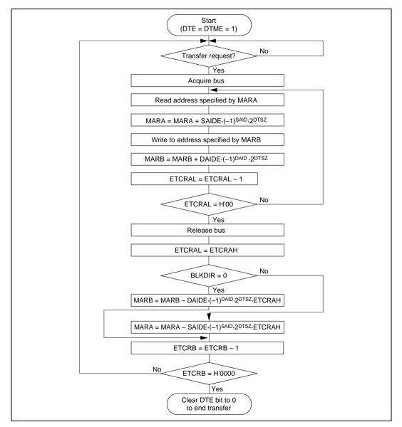
Figure 7.15 Operation Flow in Block Transfer Mode
