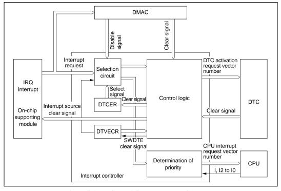
Figure 5.6 DTC, DMAC, and Interrupt Controller
