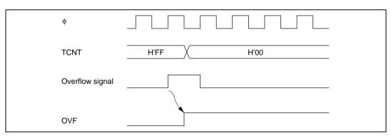
Figure 13.9 Timing of OVF Setting
