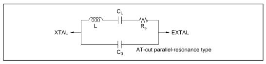
Figure 21.3 Crystal Resonator Equivalent Circuit
