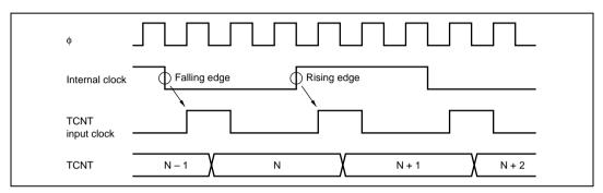
Figure 11.30 Count Timing in Internal Clock Operation
