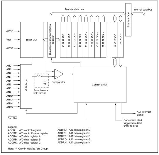
Figure 16.1 Block Diagram of A/D Converter
