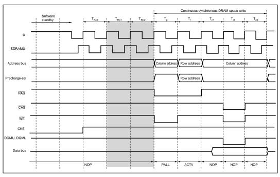
Figure 6.58 Example of Timing when Precharge Time after Self-Refreshing Is Extended by 2 States (TPCS2 to TPCS0 = H'2, TPC1 = 0, TPC0 = 0, CAS Latency 2)
