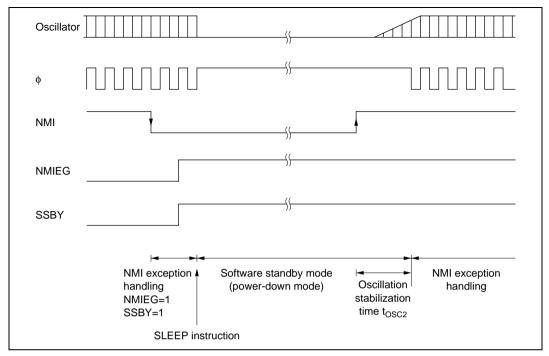
Figure 22.2 Software Standby Mode Application Example
