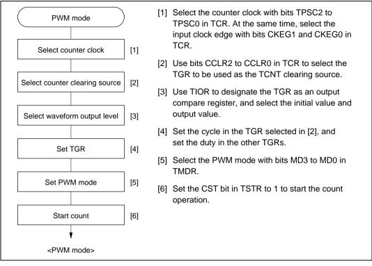
Figure 11.20 Example of PWM Mode Setting Procedure
