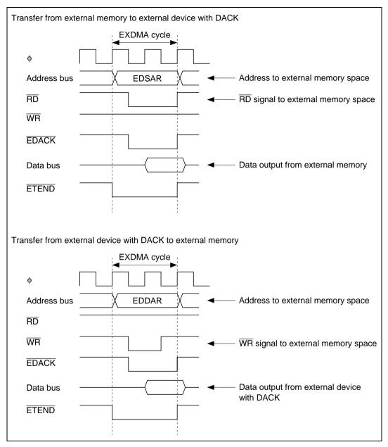
Figure 8.4 Example of Timing in Single Address Mode
