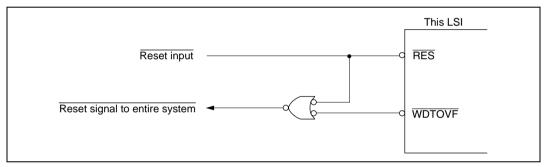
Figure 14.6 Circuit for System Reset by WDTOVF Signal (Example)
