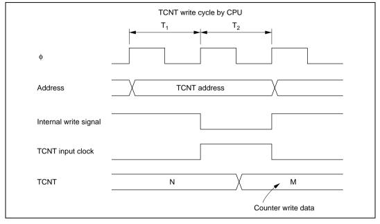
Figure 13.11 Contention between TCNT Write and Increment
