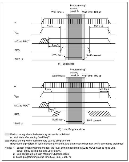
Figure 19.13 Power-On/Off Timing (H8S/2678R Group)
