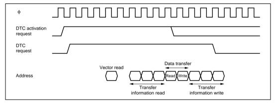
**Figure 9.9 DTC Operation Timing (Example in Normal Mode or Repeat Mode)**
