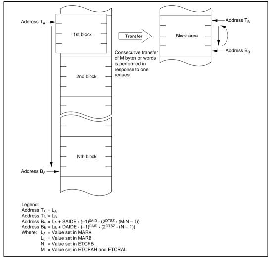
Figure 7.13 Operation in Block Transfer Mode (BLKDIR = 0)
