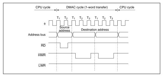
Figure 7.17 Example of DMA Transfer Bus Timing
