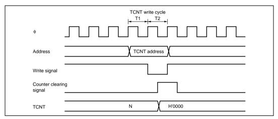
Figure 11.45 Contention between TCNT Write and Clear Operations
