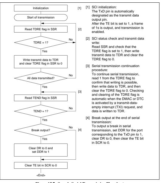
Figure 15.7 Sample Serial Transmission Flowchart
