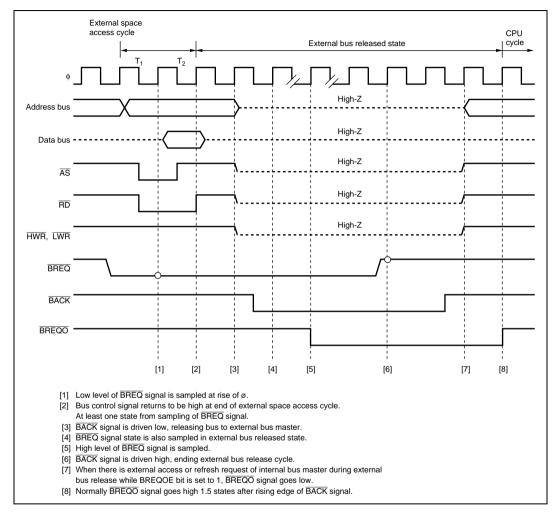
Figure 6.84 Bus Released State Transition Timing
