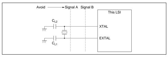
Figure 21.6 Note on Board Design for Oscillation Circuit
