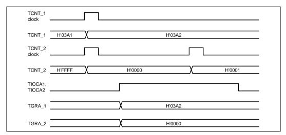
Figure 11.18 Example of Cascaded Operation (1)
