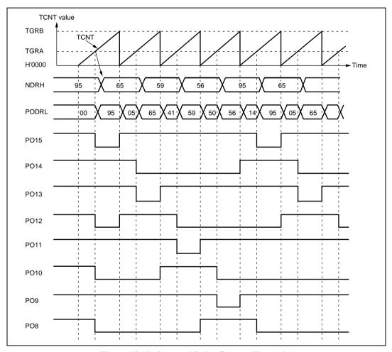
Figure 12.10 Inverted Pulse Output (Example)
