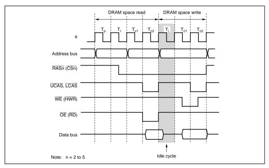
Figure 6.81 Example of Timing for Idle Cycle Insertion in Case of Consecutive Read and Write Accesses to DRAM Space in RAS Down Mode
