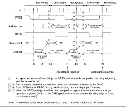
Figure 7.30 Example of DREQ Pin Falling Edge Activated Single Address Mode Transfer
