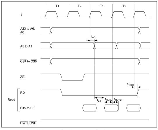
Figure 24.12 Burst ROM Access Timing: One-State Burst Access
