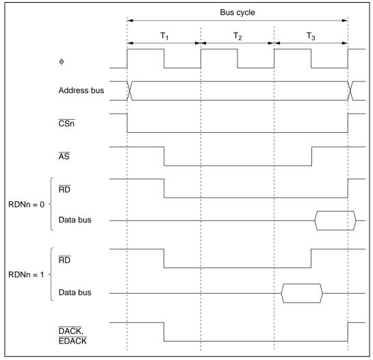
Figure 6.19 Example of Read Strobe Timing
