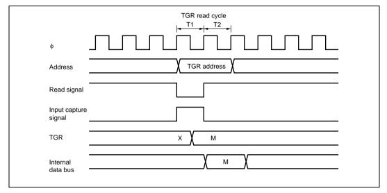
Figure 11.49 Contention between TGR Read and Input Capture
