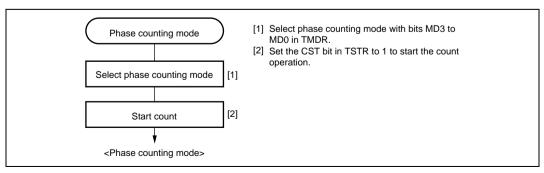
Figure 11.24 Example of Phase Counting Mode Setting Procedure
