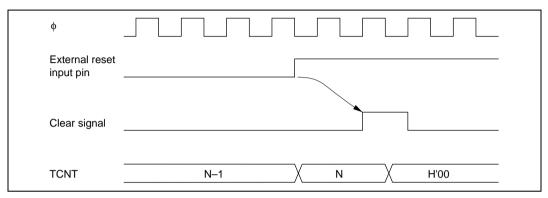
Figure 13.8 Timing of Clearance by External Reset
