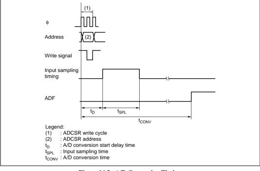
Figure 16.2 A/D Conversion Timing
