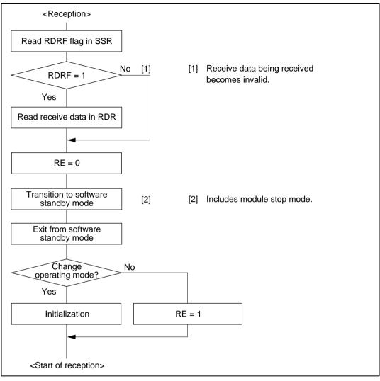
Figure 15.39 Sample Flowchart for Mode Transition during Reception
