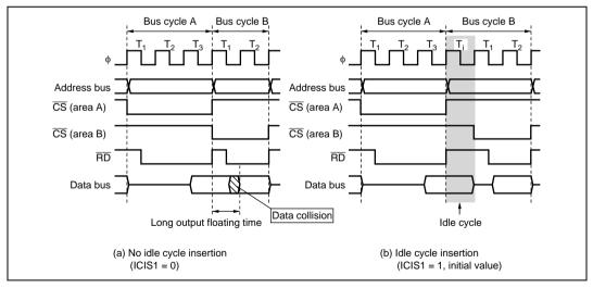
Figure 6.65 Example of Idle Cycle Operation (Consecutive Reads in Different Areas)
