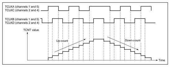
Figure 11.25 Example of Phase Counting Mode 1 Operation
