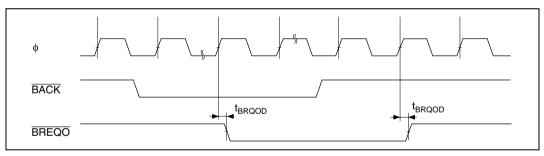
Figure 24.25 External Bus Request Output Timing
