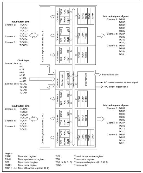
Figure 11.1 Block Diagram of TPU
