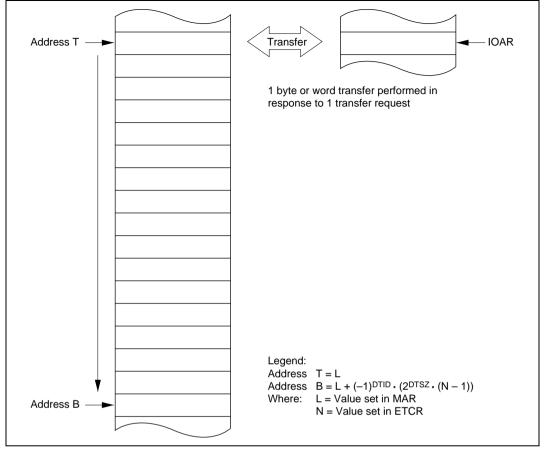
Figure 7.3 Operation in Sequential Mode
