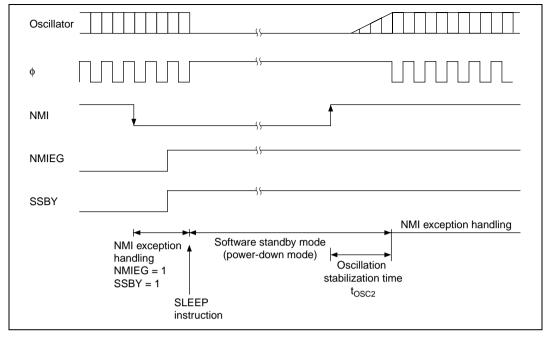
Figure 24.4 (2) Oscillation Stabilization Timing
