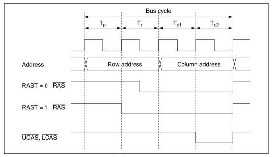
Figure 6.4 RAS Signal Assertion Timing (2-State Column Address Output Cycle, Full Access)
