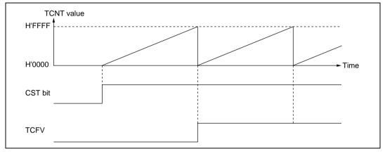
Figure 11.3 Free-Running Counter Operation
