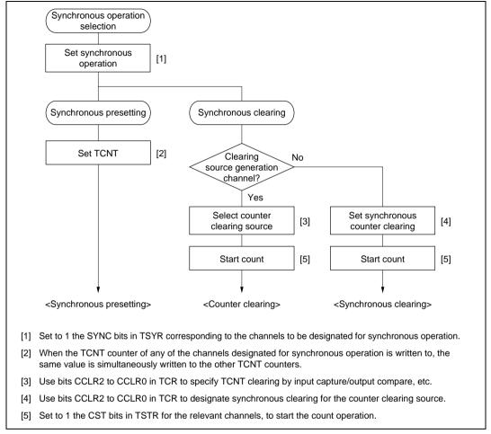
Figure 11.10 Example of Synchronous Operation Setting Procedure
