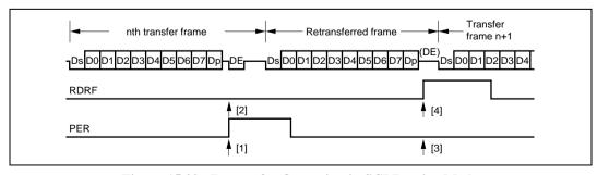
Figure 15.29 Retransfer Operation in SCI Receive Mode
