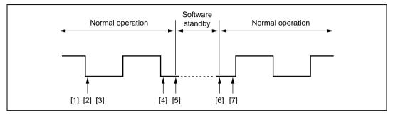
Figure 15.32 Clock Halt and Restart Procedure
