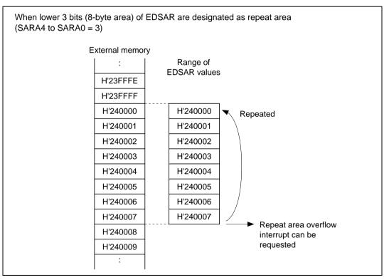
Figure 8.9 Example of Repeat Area Function Operation
