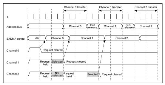
Figure 8.13 Example of Channel Priority Timing
