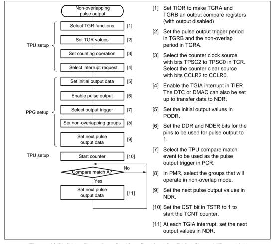
Figure 12.8 Setup Procedure for Non-Overlapping Pulse Output (Example)
