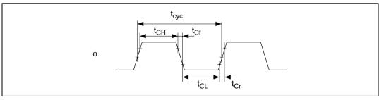
Figure 24.2 System Clock Timing
