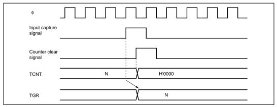
Figure 11.35 Counter Clear Timing (Input Capture)
