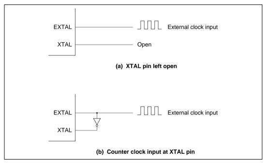
Figure 21.4 External Clock Input (Examples)
