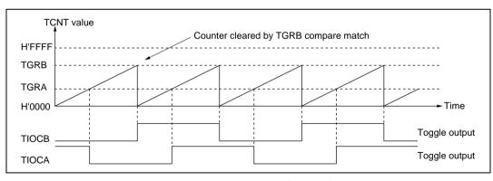
Figure 11.7 Example of Toggle Output Operation
