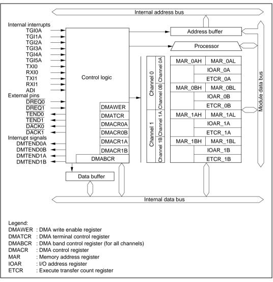
Figure 7.1 Block Diagram of DMAC
