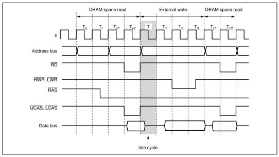
Figure 6.77 Example of Idle Cycle Operation after DRAM Access (Write after Read) (IDLC = 0, RAST = 0, CAST = 0)
