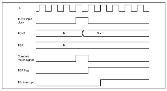
Figure 11.38 TGI Interrupt Timing (Compare Match)
