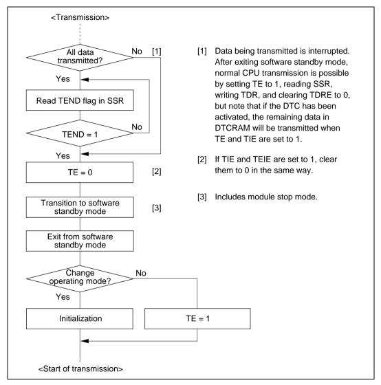
Figure 15.36 Sample Flowchart for Mode Transition during Transmission
