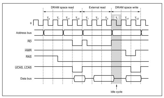
Figure 6.71 Example of Idle Cycle Operation in RAS Down Mode (Write after Read) (IDLC = 0, RAST = 0, CAST = 0)
