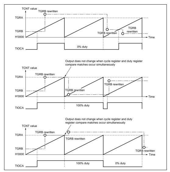
Figure 11.23 Example of PWM Mode Operation (3)
