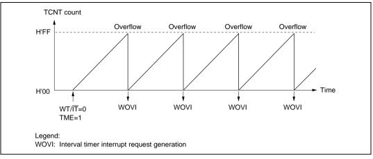
Figure 14.3 Operation in Interval Timer Mode
