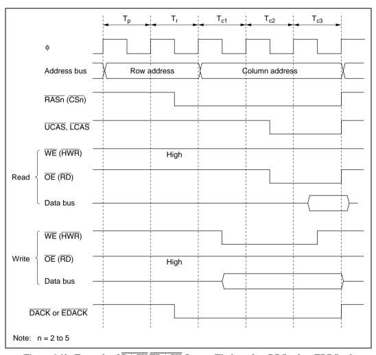
Figure 6.42 Example of  $\overline{DACK}/\overline{EDACK}$  Output Timing when DDS = 0 or EDDS = 0 (RAST = 0, CAST = 1)
