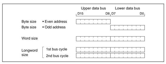
Figure 6.9 Access Sizes and Data Alignment Control (16-bit Access Space)
