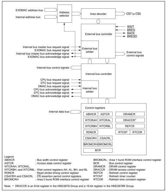
Figure 6.1 Block Diagram of Bus Controller
