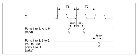
Figure 24.34 I/O Port Input/Output Timing
