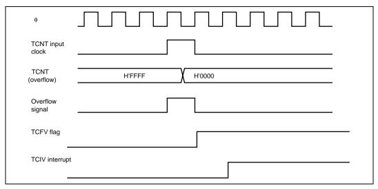
Figure 11.40 TCIV Interrupt Setting Timing
