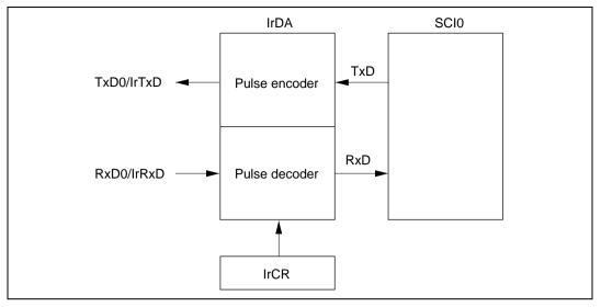
Figure 15.33 Block Diagram of IrDA
