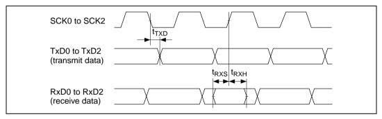
Figure 24.43 SCI Input/Output Timing: Synchronous Mode
