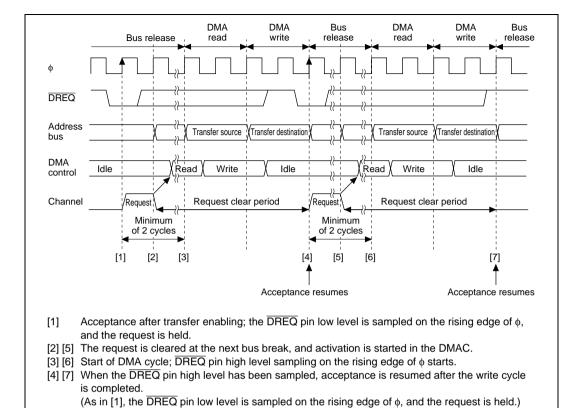
Note: In write data buffer mode, bus breaks from [2] to [7] may be hidden, and not visible.
