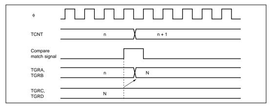
**Figure 11.36 Buffer Operation Timing (Compare Match)**
