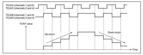
Figure 11.28 Example of Phase Counting Mode 4 Operation
