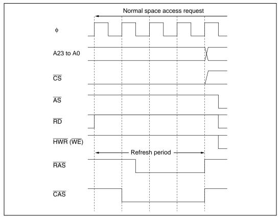
Figure 6.38 Example of CBR Refresh Timing (CBRM = 1)
