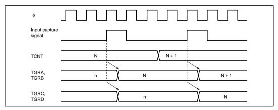
**Figure 11.37 Buffer Operation Timing (Input Capture)**
