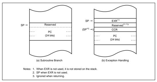
Figure 2.4 Stack Structure in Advanced Mode
