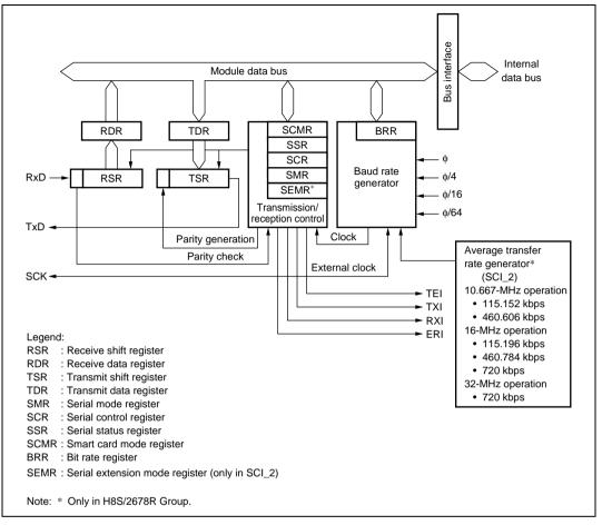
Figure 15.1 Block Diagram of SCI
