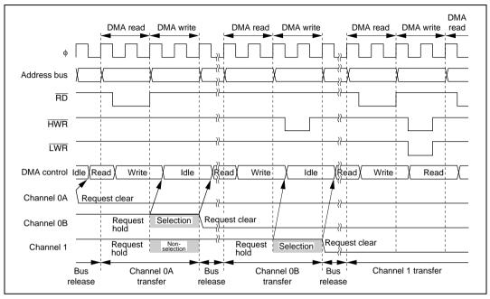
Figure 7.34 Example of Multi-Channel Transfer
