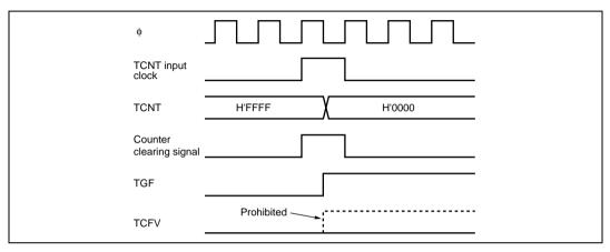
Figure 11.52 Contention between Overflow and Counter Clearing
