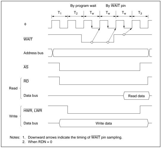
Figure 6.18 Example of Wait State Insertion Timing
