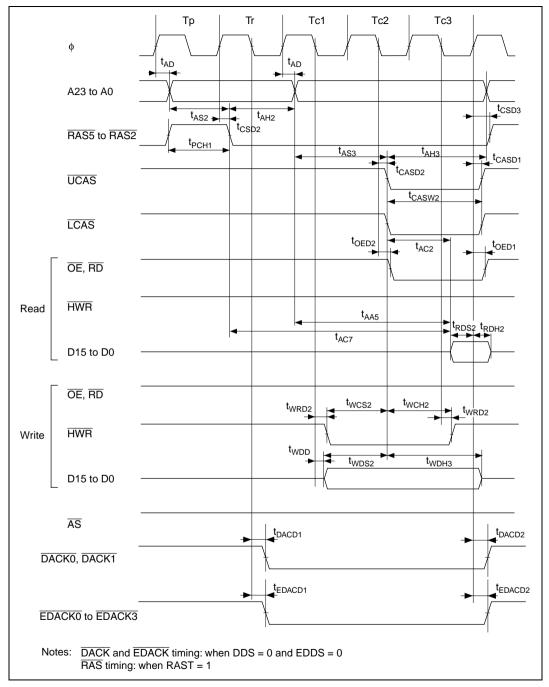
Figure 24.17 DRAM Access Timing: Three-State Access (RAST = 1)
