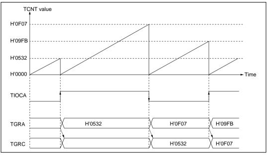
Figure 11.16 Example of Buffer Operation (2)
