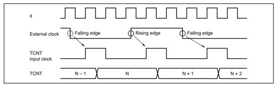
Figure 11.31 Count Timing in External Clock Operation
