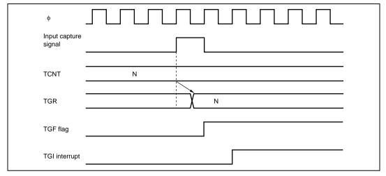
Figure 11.39 TGI Interrupt Timing (Input Capture)
