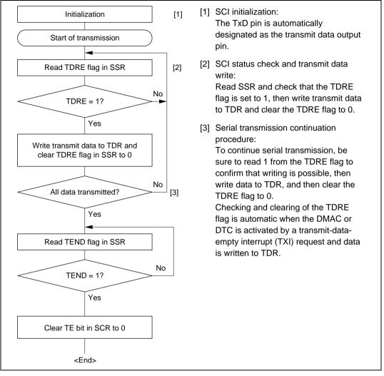
Figure 15.17 Sample Serial Transmission Flowchart
