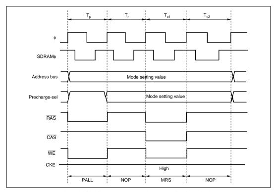
Figure 6.59 Synchronous DRAM Mode Setting Timing
