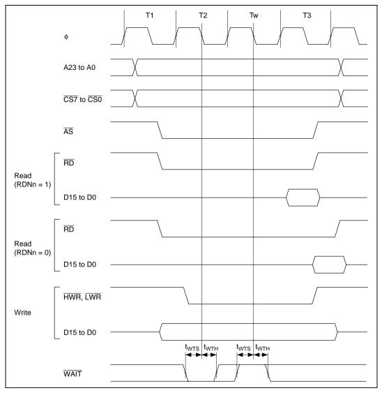
Figure 24.9 Basic Bus Timing: Three-State Access, One Wait
