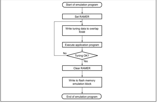
Figure 19.8 Flowchart for Flash Memory Emulation in RAM
