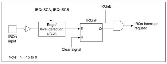
Figure 5.2 Block Diagram of Interrupts IRQ15 to IRQ0
