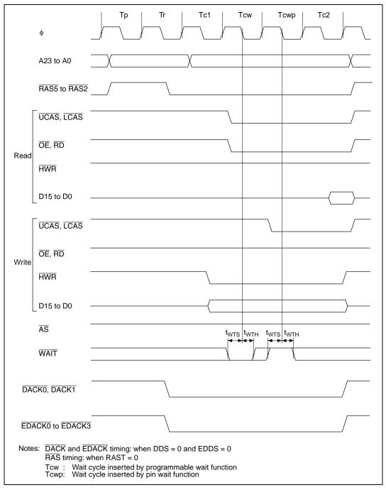
Figure 24.15 DRAM Access Timing: Two-State Access, One Wait
