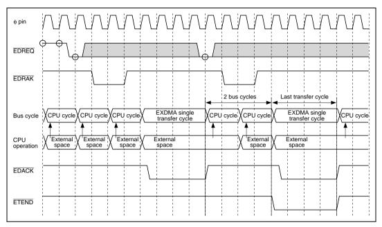
Figure 8.36 External Request/Cycle Steal Mode/Normal Transfer Mode (CPU Cycles/Single Address Mode/Low Level Sensing)
