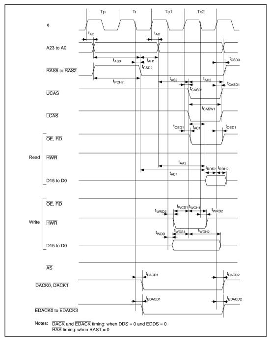
Figure 24.14 DRAM Access Timing: Two-State Access
