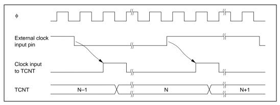
Figure 13.4 Count Timing for External Clock Input
