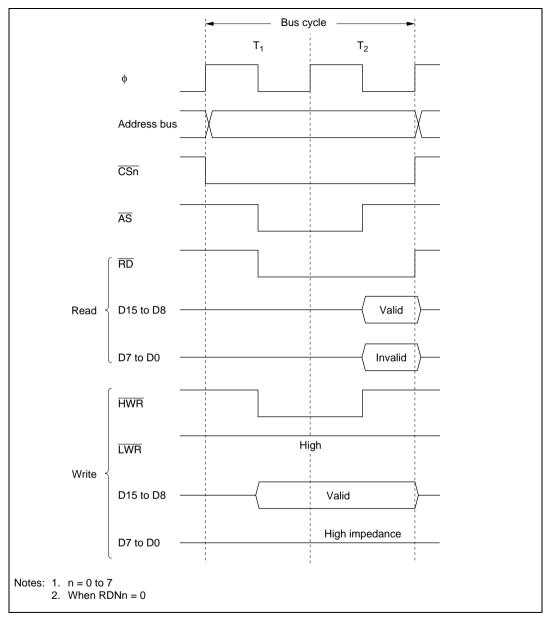
Figure 6.10 Bus Timing for 8-Bit, 2-State Access Space
