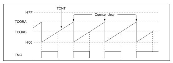
Figure 13.2 Example of Pulse Output
