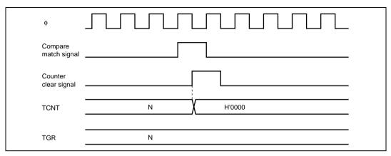
Figure 11.34 Counter Clear Timing (Compare Match)
