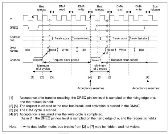
Figure 7.24 Example of DREQ Pin Low Level Activated Normal Mode Transfer
