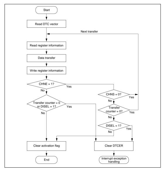
Figure 9.4 Flowchart of DTC Operation
