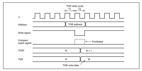
Figure 11.47 Contention between TGR Write and Compare Match
