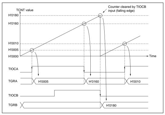
Figure 11.9 Example of Input Capture Operation
