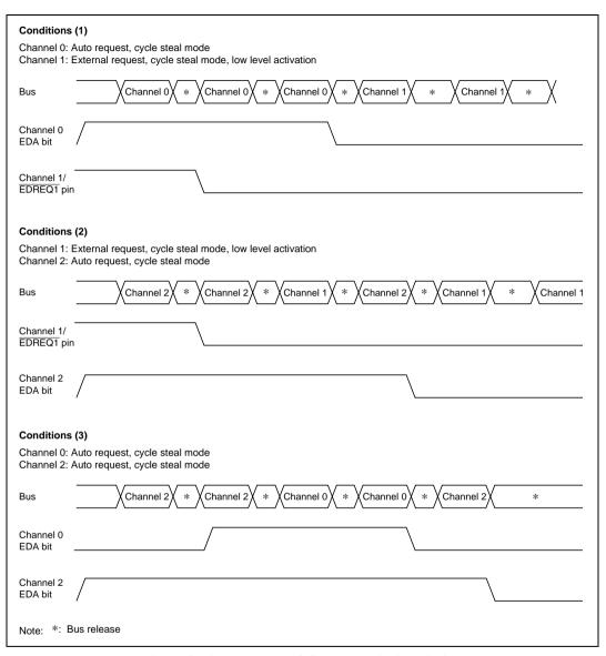
Figure 8.14 Examples of Channel Priority Timing
