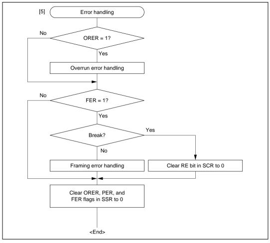
Figure 15.13 Sample Multiprocessor Serial Reception Flowchart (2)
