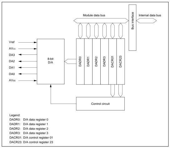
Figure 17.1 Block Diagram of D/A Converter
