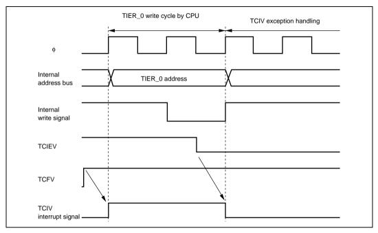
Figure 5.7 Contention between Interrupt Generation and Disabling
