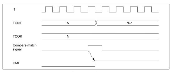
Figure 13.5 Timing of CMF Setting
