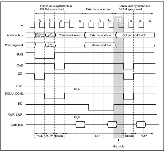
Figure 6.73 Example of Idle Cycle Operation in RAS Down Mode (Read in Different Area) (IDLC = 0, CAS Latency 2)
