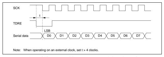
Figure 15.35 Example of Synchronous Transmission Using DTC
