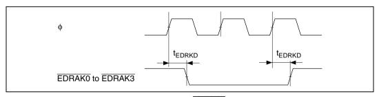
Figure 24.33 EXDMAC EDRAK Output Timing
