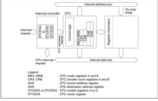
Figure 9.1 Block Diagram of DTC
