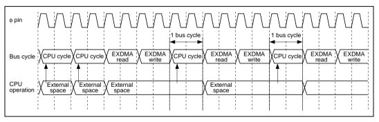
Figure 8.32 Auto Request/Burst Mode/Normal Transfer Mode (CPU Cycles/Dual Address Mode/BGUP = 1)
