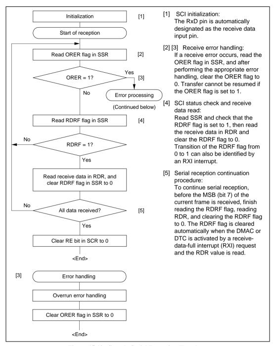
Figure 15.19 Sample Serial Reception Flowchart
