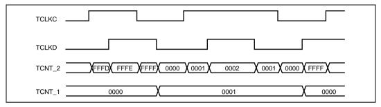
Figure 11.19 Example of Cascaded Operation (2)
