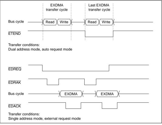
Figure 8.7 Examples of Timing in Normal Transfer Mode
