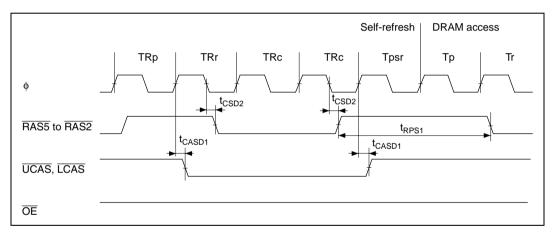
Figure 24.23 Self-Refresh Timing (Return from Software Standby Mode: RAST = 1)
