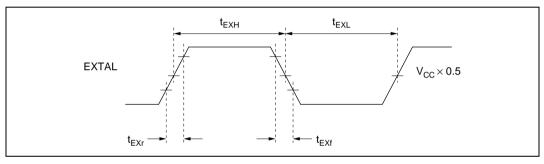
Figure 21.5 External Clock Input Timing
