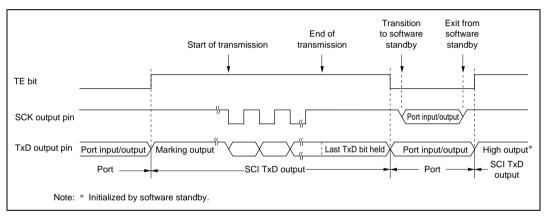
Figure 15.38 Port Pin States during Mode Transition (Internal Clock, Synchronous Transmission)
