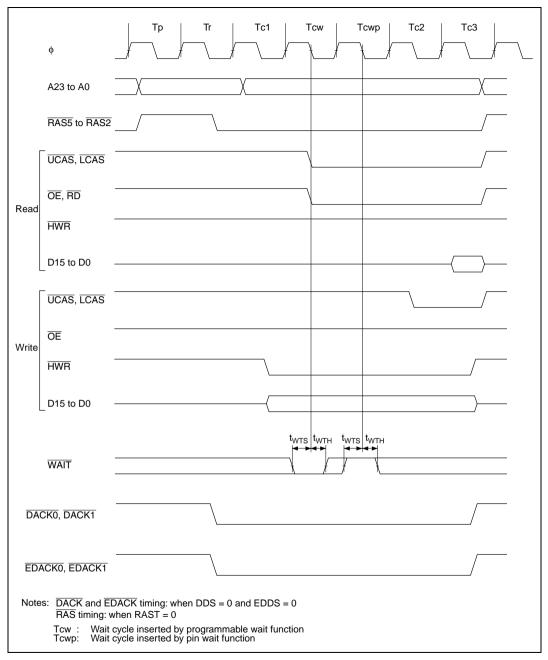
Figure 24.18 DRAM Access Timing: Three-State Access, One Wait
