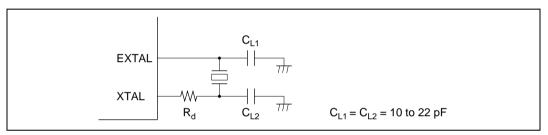
Figure 21.2 Connection of Crystal Resonator (Example)
