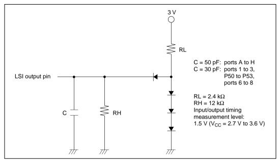
Figure 24.1 Output Load Circuit
