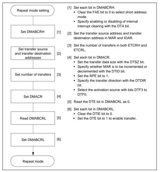
Figure 7.8 Example of Repeat Mode Setting Procedure
