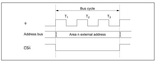
Figure 6.7  $\overline{CSn}$  Signal Output Timing (n = 0 to 7)
