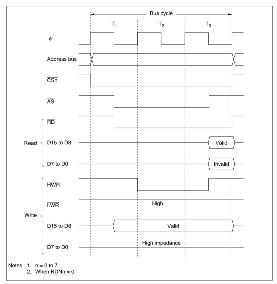
Figure 6.11 Bus Timing for 8-Bit, 3-State Access Space
