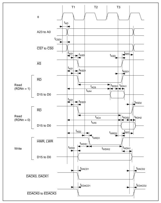
Figure 24.8 Basic Bus Timing: Three-State Access
