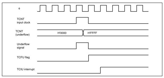
Figure 11.41 TCIU Interrupt Setting Timing
