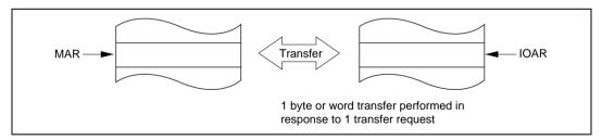
Figure 7.5 Operation in Idle Mode
