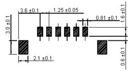
**PCB Layout Surface Mounting**
