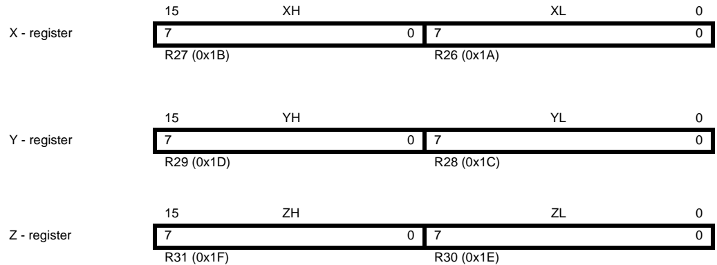
Figure 5. The X-, Y-, and Z-Registers
