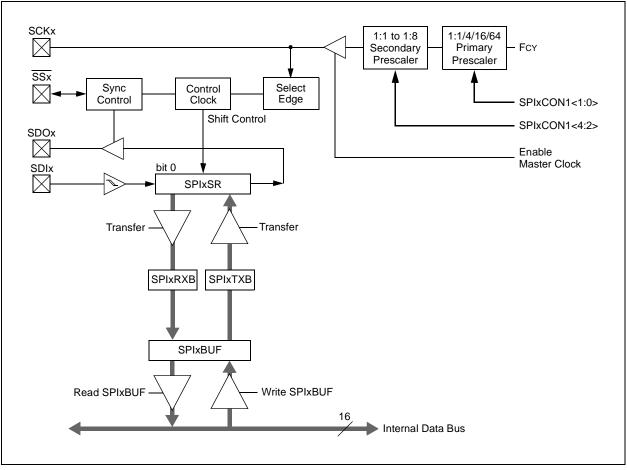
**Note:** The dsPIC30F1010/2020 devices do not contain the SS1 pin. Therefore, the Slave Select and Frame Sync features cannot be used on these devices. These features are available on the dsPIC30F2023.
