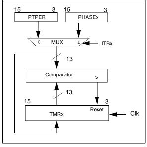
Normally, the Primary Time Base (PTMR) provides synchronization control to the individual timer/counters so they count in lock-step unison.
