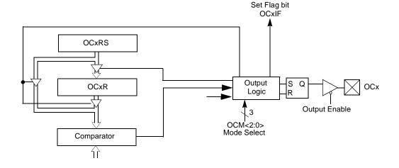
**Note:** Where 'x' is shown, reference is made to the registers associated with the respective output compare channels 1 and 2.
