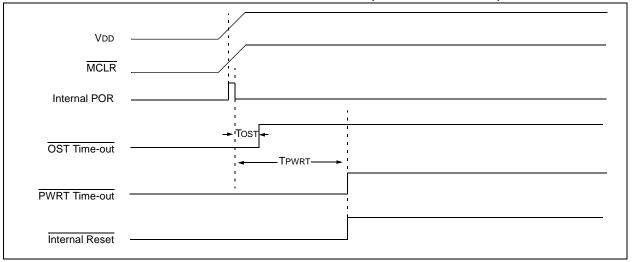
FIGURE 18-9: TIME-OUT SEQUENCE ON POWER-UP (MCLR NOT TIED TO VDD): CASE 1
