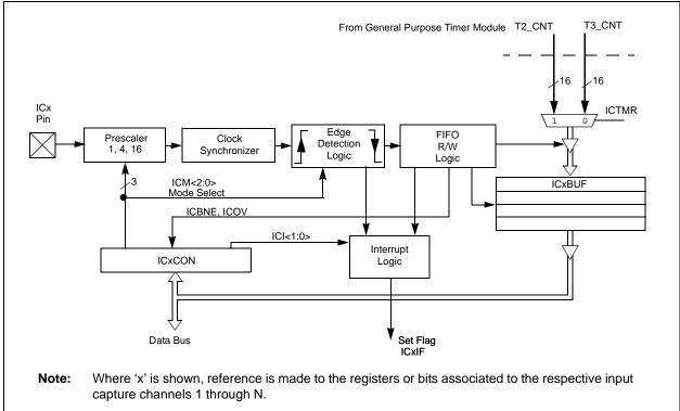
**INPUT CAPTURE MODE BLOCK DIAGRAM**
