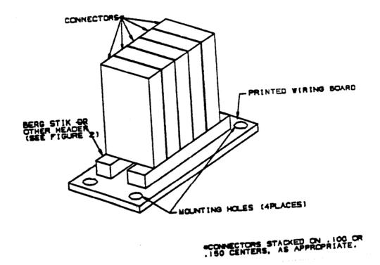
**FIGURE 4 - MOUNTING FOR STOCK/VIBRATION**
