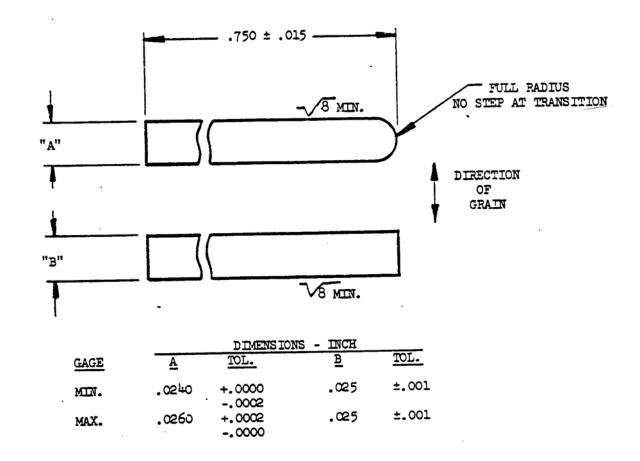
Material: Shim stock; grind to width and break edges; do not polish working surface.
