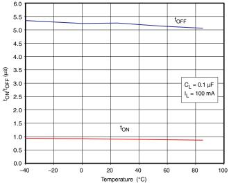
Figure 12. t<sub>rise</sub> (TPS22903/4) / t<sub>fall</sub> (TPS22903) vs Temperature (V<sub>IN</sub> = 3.3 V)
