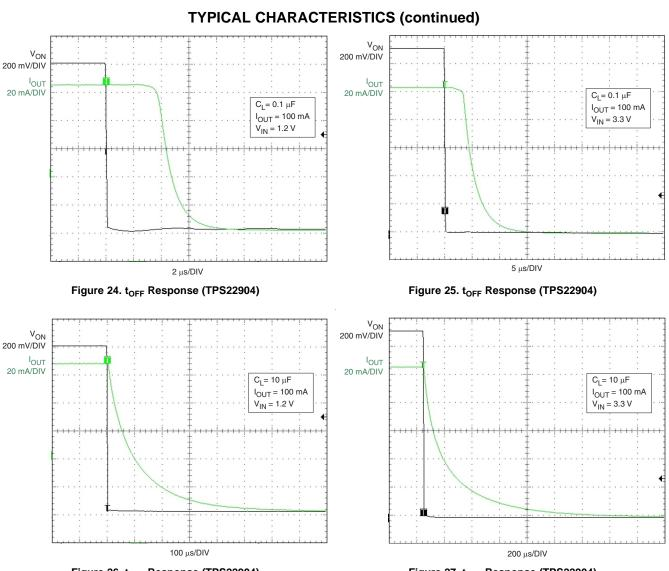
Figure 26. t<sub>OFF</sub> Response (TPS22904)
