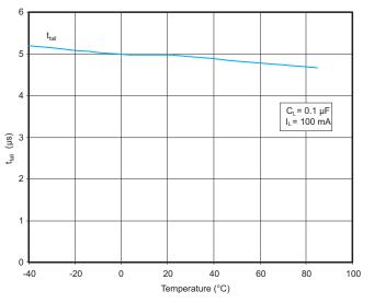
Figure 14.  $t_{fall}$  (TPS22904) vs Temperature (V<sub>IN</sub> = 3.3 V)
