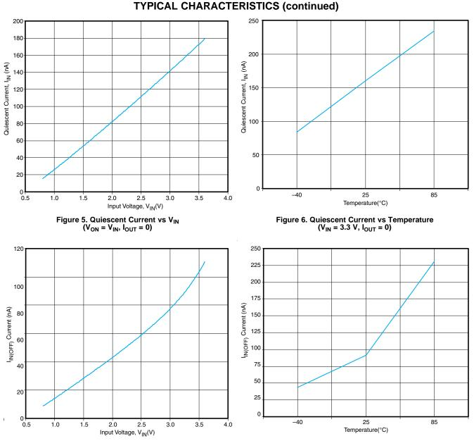
Figure 7.  $I_{IN(OFF)}$  vs  $V_{IN}$  ( $V_{ON} = 0$  V)
