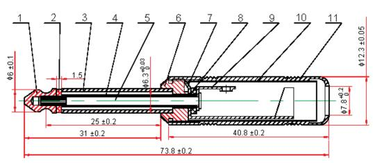
The terminal plating silver, thickness 0.5µm (SOLDER).
