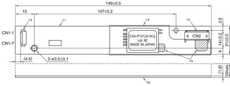
\*1Substrate(PWB: Printed wiring board): Inflammable material UL 94V-0(FR-4 or CEM-3)
