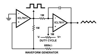
NOTE: Since the output range swings exactly from rail to rail, frequency and duty cycle are virtually independent of power supply variations.
