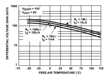
FIGURE 12. LARGE SIGNAL DIFFERENTIAL VOLTAGE GAIN vs FREE-AIR TEMPERATURE
