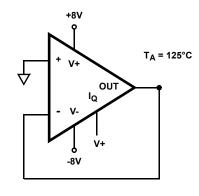
FIGURE 6. BURN-IN AND LIFE TEST CIRCUIT
