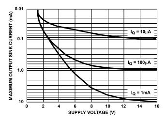
FIGURE 22. OUTPUT SINK CURRENT vs SUPPLY VOLTAGE
