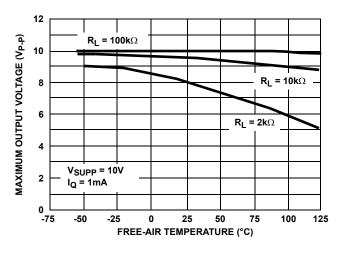
FIGURE 20. OUTPUT VOLTAGE vs FREE-AIR TEMPERATURE
