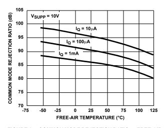
FIGURE 14. COMMON MODE REJECTION RATIO vs FREE-AIR TEMPERATURE
