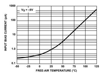
FIGURE 11. INPUT BIAS CURRENT vs TEMPERATURE
