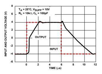
FIGURE 24. VOLTAGE FOLLOWER LARGE SIGNAL PULSE RESPONSE ( $I_Q = 1 \text{mA}$ )
