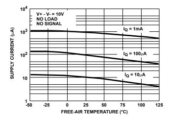
FIGURE 10. SUPPLY CURRENT PER AMPLIFIER vs FREE-AIR TEMPERATURE
