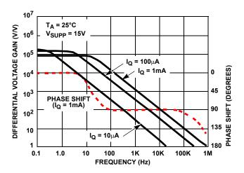
FIGURE 13. LARGE SIGNAL FREQUENCY RESPONSE
