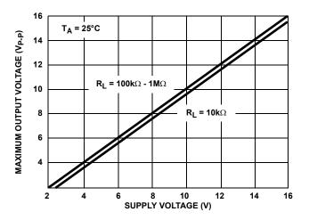
FIGURE 19. OUTPUT VOLTAGE vs SUPPLY VOLTAGE
