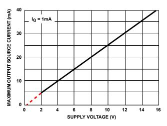
FIGURE 21. OUTPUT SOURCE CURRENT vs SUPPLY VOLTAGE
