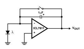
NOTE: Low leakage currents allow integration times up to several hours.
