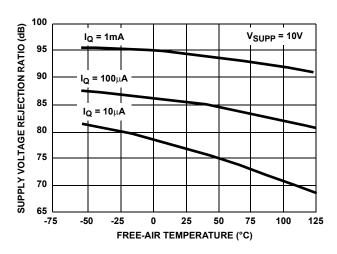
FIGURE 15. POWER SUPPLY REJECTION RATIO vs FREE-AIR TEMPERATURE
