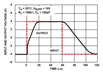
FIGURE 25. VOLTAGE FOLLOWER LARGE SIGNAL PULSE RESPONSE ( $I_Q = 100 \mu A$ )
