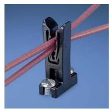
Secures wire ends with or without terminations while harness is being fabricated. Wires can be easily added or removed from the top, but will hold the wire from axial movement. Used with #28 thru #16 AWG wires. Two mounting slots .16 (4.1) for #8 (M4) screws.
