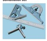
The square and centre heads are of hardened steel. Protractor head is reversible and is graduated 0° to 180° in both directions. All heads have blue stove enamelled hammer finish with accurately ground working surfaces. The 300mm/12in blade is fully tempered and hardened. Satin chrome finish gives exceptional clarity to the very fine graduations and resists abrasion.
