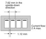
**Note:** The space between each relay required for heat radiation may vary with operating conditions. Contact your OMRON representative for details.
