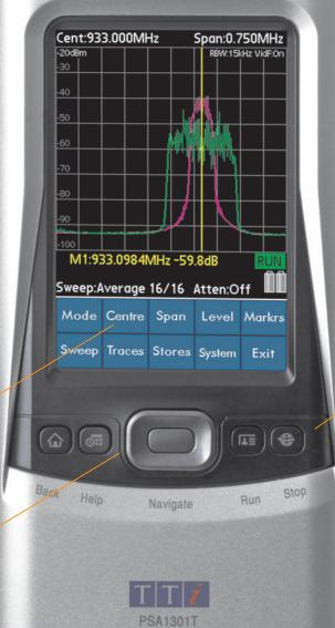
1.3GHz RF Spectrum Analyzer
