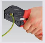
Third step: when greater handforce is required, such as e.g. when crimping insulated connectors 6.0 mm<sup>2</sup>, two hand operation is possible by the longer handles
