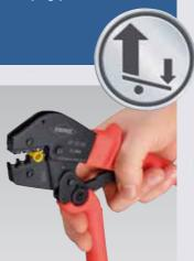
First step: move the handle with two fingers only until both jaws touch the connector to be crimped
