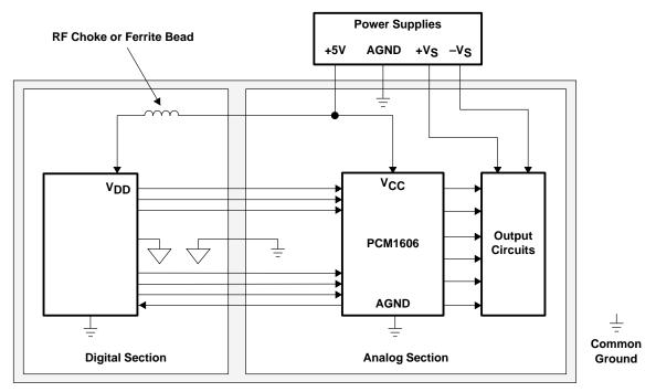
Figure 33. Single-Supply PCB Layout
