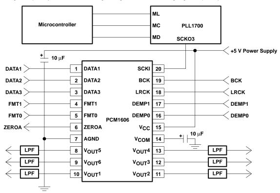
Figure 28. Basic Connection Diagram
