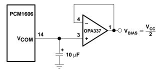
Figure 8. Biasing External Circuits Using the  $V_{\mbox{COM}}$  Pin
