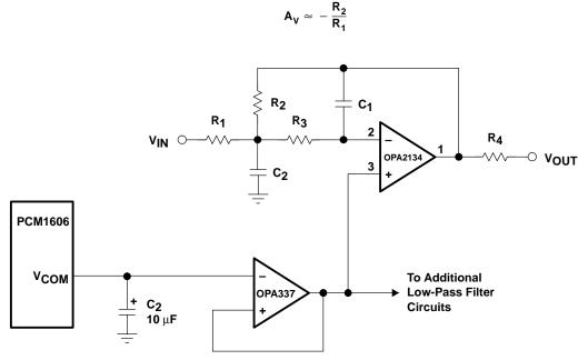
Figure 31. Single-Supply Filter Circuit
