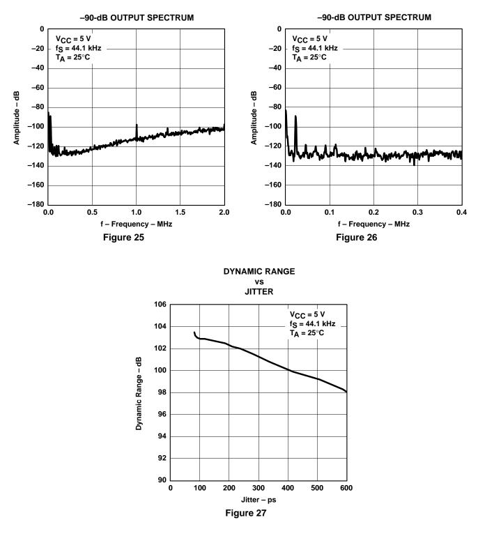
All specifications at  $T_A = 25^{\circ}C$ ,  $V_{CC} = 5$  V,  $f_S = 44.1$  kHz, system clock = 384  $f_S$  and 24-bit data, unless otherwise noted.
