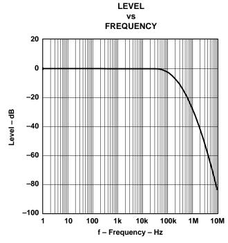
Figure 7. Output Filter Frequency Response
