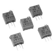
The Model 64 is a small size trimmer - 3/8" x 3/8" x 3/16" - answering PC board mounting requirements. Five versions are available which differ by the position of the control screw in relation to the PC board plane and by the spacing of the terminals. Excellent operational stability is provided by the use of a cermet element.
