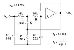
Figure 14. Active High-Q Notch Filter
