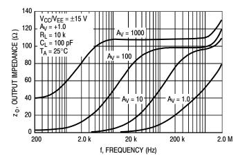
Figure 8. Output Impedance and Frequency
