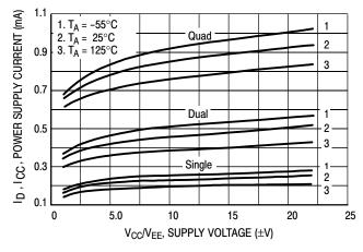
Figure 9. Supply Current versus Supply Voltage
