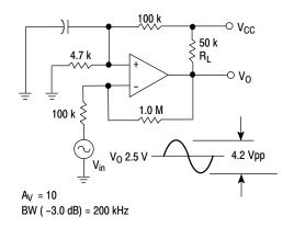
Figure 12. DC Coupled Inverting Amplifier
