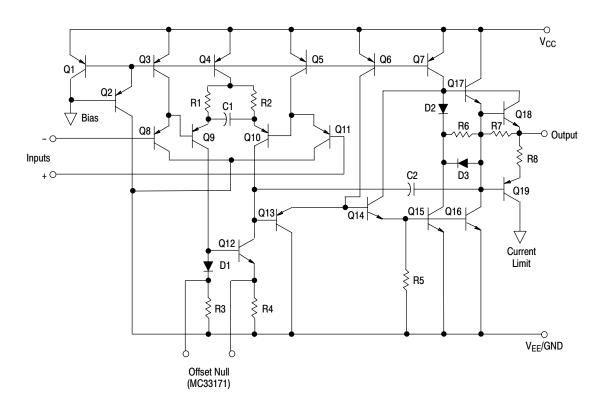
Figure 1. Representative Schematic Diagram (Each Amplifier)
