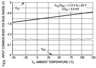
Figure 2. Input Common Mode Voltage Range versus Temperature
