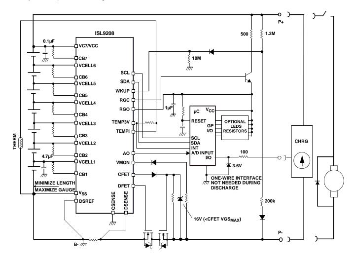
FIGURE 15. 7-CELL APPLICATION CIRCUIT INTEGRATED CHARGE/DISCHARGE
