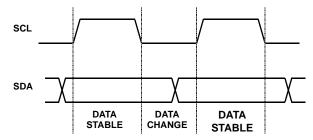
FIGURE 9. VALID DATA CHANGES ON I<sup>2</sup>C BUS
