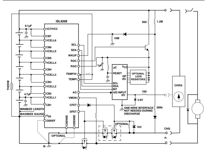
FIGURE 16. 7-CELL APPLICATION CIRCUIT SEPARATE CHARGE/DISCHARGE
