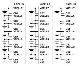
Note: Multiple cells can be connected in parallel
