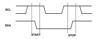
FIGURE 10. I<sup>2</sup>C START AND STOP BITS
