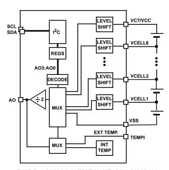
FIGURE 6. ANALOG OUTPUT MONITORING DIAGRAM
