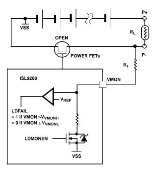
FIGURE 4. LOAD MONITOR CIRCUIT
