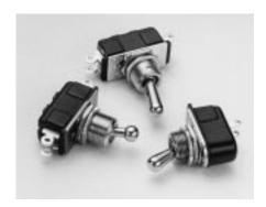
The 110/216-Series toggle switches utilize a quick-make, quick-break contact mechanism and are available in both single and double pole. These switches are 125-250 volts AC/DC rated and suitable for shallow back panel applications. They are available in a range of circuits, terminations and bushing/toggle configurations.
