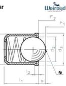
Material Body: stainless steel 1.4305 or Delrin blue. Ball: stainless steel, hardened or Delrin white (POM). Spring: stainless steel. Technical Notes Used for locating, applying pressure or lifting off. spring loads \* = statistical average values.
