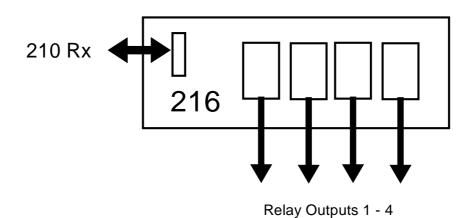
This DIN Rail module connects directly to the 210Rx and provides four relay outputs rated at 230Vac providing 12A peak and 5A continuous current rating. The only connections required are
