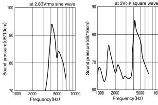
\* The frequency characteristic changes depending on the case shape and the installation method.
