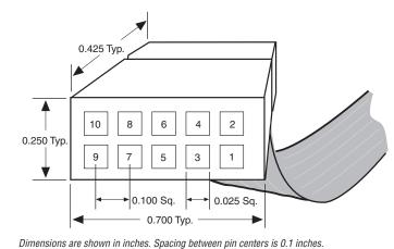
Figure 2–2. USB-Blaster 10-Pin Female Plug Dimensions
