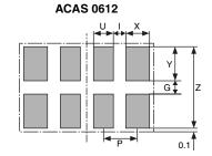
Dimensions in mm ☐ limits for solder resistance
