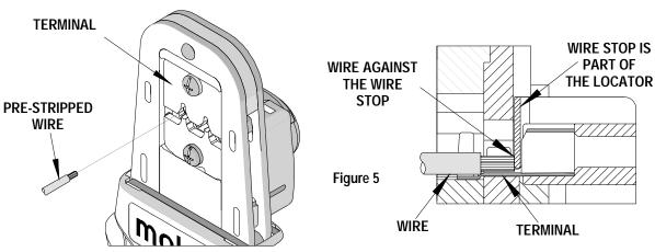
Note: The tamper proof ratchet action will not release the tool until it has been fully closed.
