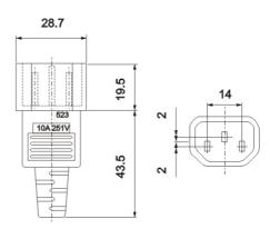
End 1: IEC Cold Connector (C13) black Fuse: n/a Lead: 2,00mts HO5VV-F 3x1,00 black End 2: IEC Cold Connector Plug (C14) black
