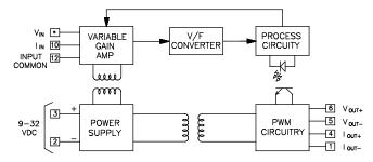
\* Terminal number is dependent on max. input voltage.
