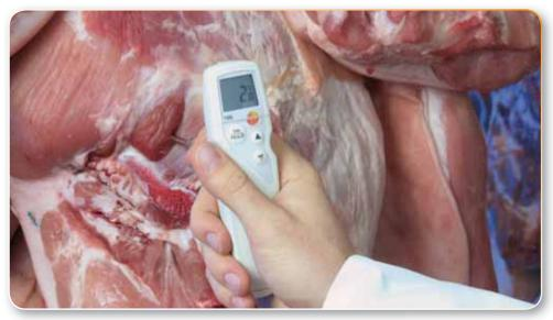
Robust hand-held T-bar thermometer, with interchangeable measurement tips, for control measurements in abattoirs, refrigerated storerooms and meat processing.
