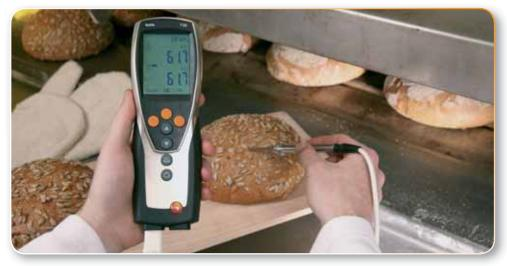
Highly versatile, multi-channel thermometer with logging ability and location management. A wide range of optional probes available including Pt100, T/C Type K, T/C Type T and wireless probes.
