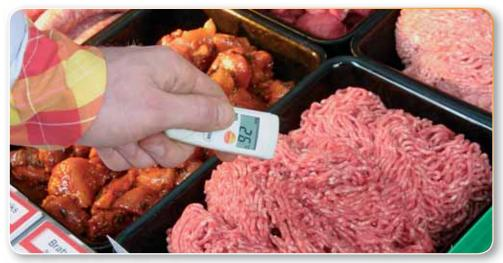
Compact infrared thermometer ideal for quick measurements at delivery, storage and hot cupboards. For quick surface and air measurements of fridge/freezers, hot cupboards and point of delivery.
