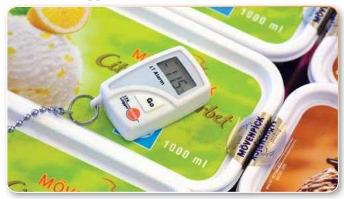
High accuracy single channel mini temperature data logger with digital display, ideal for monitoring temperature during transportation and storage.
