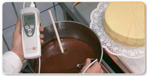
Designed for use throughout the food industry this fast and accurate thermometer can be used with both corded and optional wireless probes.
