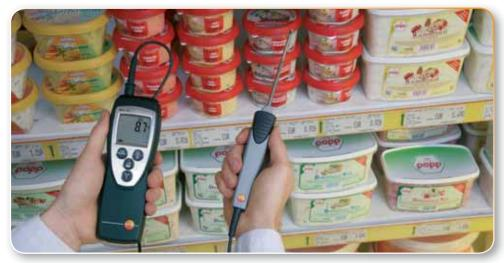
Designed for use throughout the food processing and service industry, this versatile thermometer can be used with both corded and optional wireless probes.
