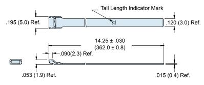
**The 600-083 Extended Length Micro-Band** is precision constructed of 300 Series SST/Passivate, and designed for use with the 600-061 Hand Banding Tool or the 600-068 Pneumatic Banding Tool. Double-wrapped bands will accommodate diameters up to approximately 1.88 inches (47.8). Bands may be ordered flat (600-083), or precoiled (600-083-1). Bands come bagged and tagged in quantities from 1 to 100.
