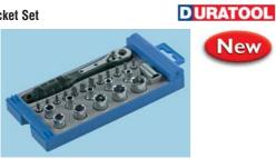
Manufactured from chrome vanadium steel and supplied in a blow moulded case Contents: Sockets ¼": 4, 5, 5.5, 6, 8, 9, 10, 11, 12, 13 mm Slotted: 4, 5, 6 mm Phillips: PH1, PH2 Pozidriv: PZ1, PZ2 Torx: T10, T15, T20 Hex: 4 mm 1 x ¼" Screwdriver bit holder, 1 x Drive socket adaptor, 1 x ¼" Drive ratchet handle
