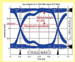
Fig. 1: Eye diagram of a 1280 MBit signal (512 Bits)
